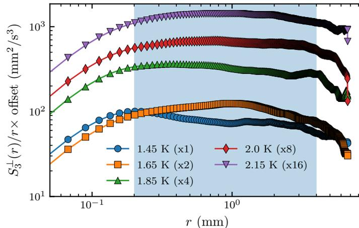
FIG. 5. Third order transverse velocity structure functions compensated by linear scaling,  $S_3^\perp(r)/r$ , plotted versus the separation distance  $r$ . Data for 300 mm/s grid velocity and 4 s decay time are shown for temperatures and offsets as indicated.
