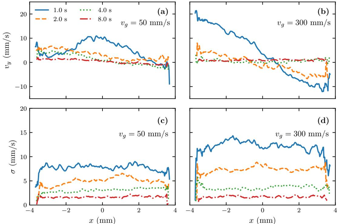
FIG. 2. (a,b) The ensemble-averaged velocity profile  $v_y(x)$  across the channel at different decay times with grid velocities  $v_g$  as indicated. (c,d) The corresponding velocity variance  $\sigma(x)$  profiles. The shown data are obtained at 1.85 K, at the indicated time instants.
