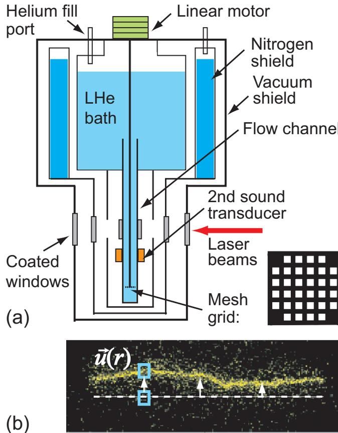
FIG. 1. (a) Schematic diagram of the experimental setup. (b) A sample image of the He<sub>2</sub>\* molecular tracer line. The white dashed line serves to demonstrate the initial location of the trace line for velocity calculations.
