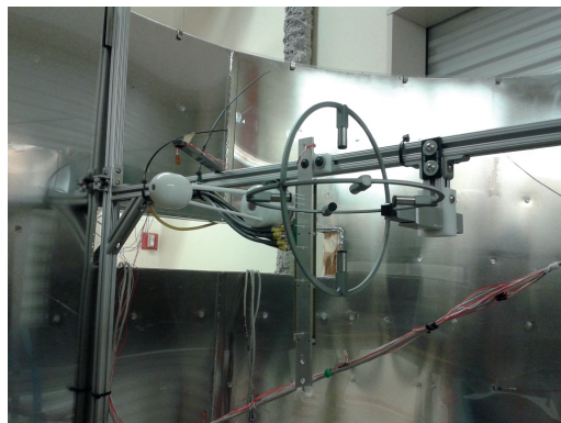
FIG. 1: Left figure: Sketch of the cloud chamber with one door being open and the cylindrical thermal panel being in place [12]. Right figure: Picture of the instrumentation inside the cylinder. The IR absorption hygrometer, the sonic anemometer, as well as the thermistor array were placed such as the distance between the instruments is as small as possible in order to avoid cross-influence between the instruments but to ensure possible cross-correlations.
