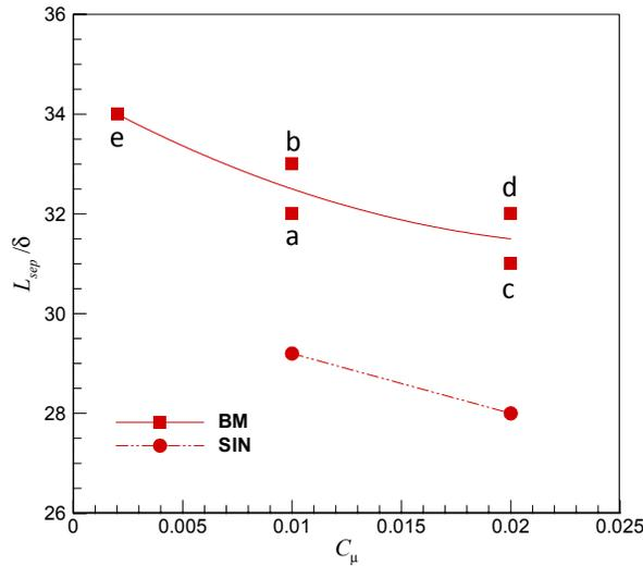
**FIG. 8.** Mean separation bubble length ( $L_{sep}$ ) versus the momentum ratio coefficient ( $C_\mu$ ). a-e: BM jet controls listed in Table 1. SIN: sinusoidal jet control case shown for the comparison. Solid line represents the quadratic best fit for the BM cases.
