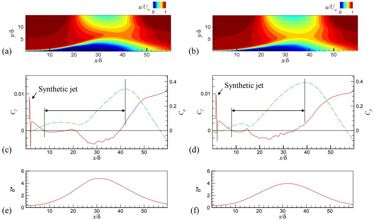
**FIG. 12.** Time-averaged fields for the control cases with the amplitude modulated synthetic jet. Streamwise velocity contours for the AM1 jet (a) and AM2 jet (b) with  $F_c^+=10$ ,  $F_m^+=1$ . Skin friction (solid line) and pressure (dashed line) coefficients profiles for the AM1 (c) and AM2 (d). Mean displacement thickness along the streamwise direction for the AM1 (e) and AM2 (f).
