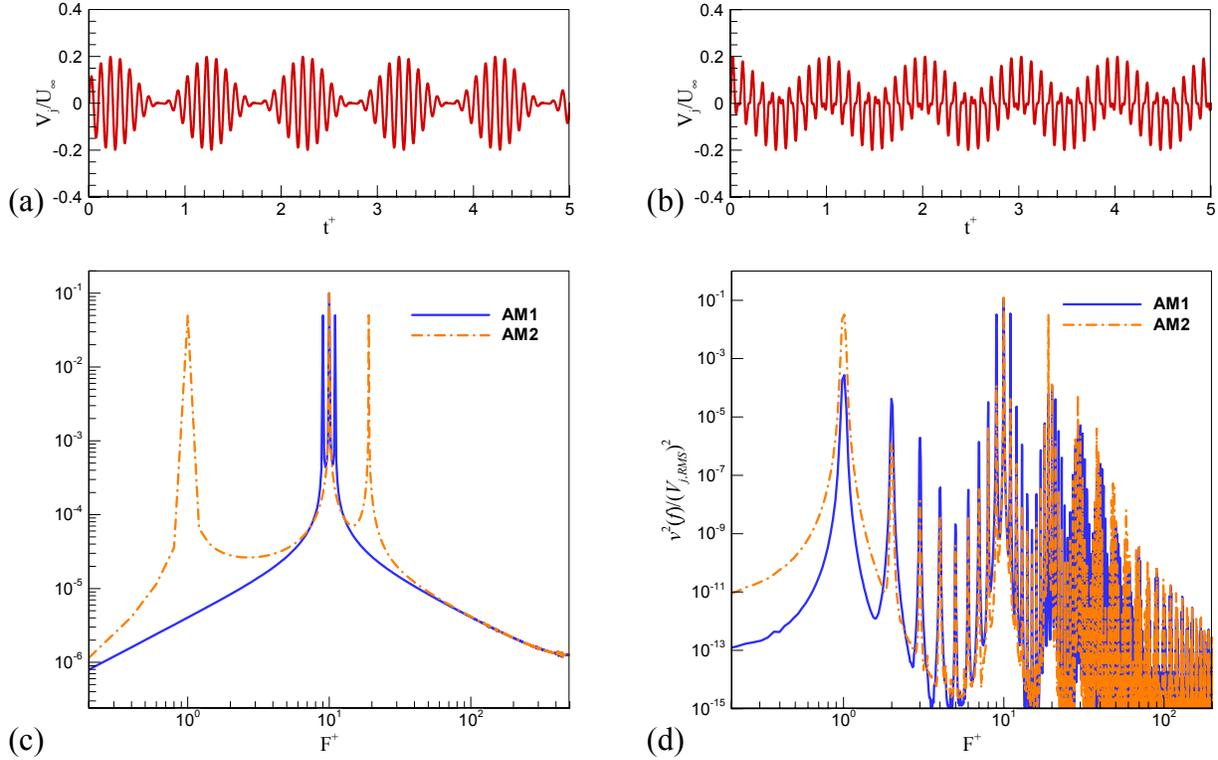
**FIG. 11. (a) Waveform of synthetic jet velocity for AM1: amplitude modulation given by Eq. 4,  $F_c^+=10$ ,  $F_m^+=1$ , and  $t^+=t \cdot f_c$ . (b) waveform for AM2: tailored amplitude modulation scheme given by Eq. 9. (c) Spectra of the synthetic jet input velocities for AM1 and AM2. (d) power spectra of vertical velocity monitored on the synthetic jet outlet port in the flow field.**
