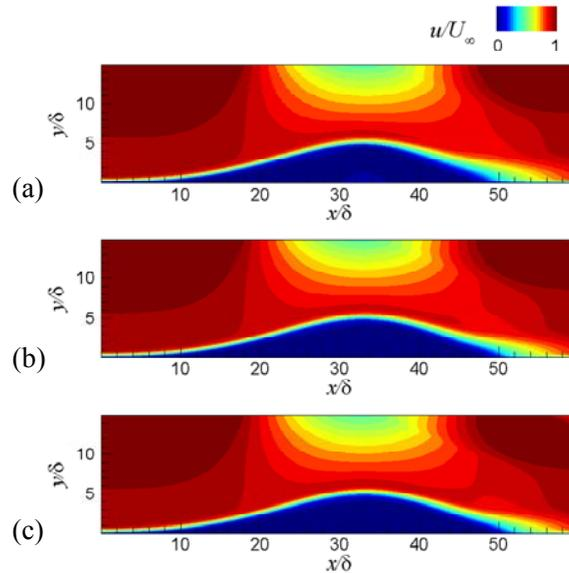
**FIG. A1. Time and spanwise averaged, streamwise velocity contours with different grid resolutions. (a) coarse ( $384 \times 96 \times 32$ ), (b) medium ( $512 \times 128 \times 32$ ), and (c) fine ( $768 \times 256 \times 32$ ) resolutions.**
