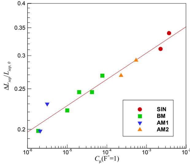
**FIG. 15. Decrease of separation bubble length ( $\Delta L_{sep}$ ) normalized by the uncontrolled length ( $L_{sep,0}$ ) versus the spectral momentum ratio coefficient at  $F^+=1$  ( $C_\mu(F^+=1)$ ). Solid line represents the best power-law fit.**
