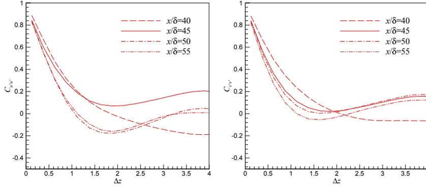
**FIG. A3. Spanwise correlation coefficients for the streamwise ( $C_{u'u'}$ ) and vertical ( $C_{v'v'}$ ) velocity fluctuations at  $y/\delta=1.5$  and various streamwise locations for baseline case with  $L_z=8\delta$  and  $N_z=32$ , ( $L_z$ : spanwise domain size,  $N_z$ : number of grid points in the spanwise direction).**
