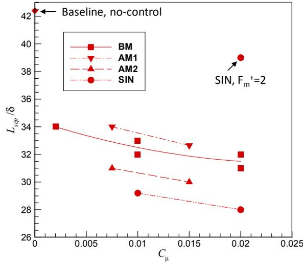
FIG. 14. Mean separation bubble length ( $L_{sep}$ ) versus the momentum ratio coefficient ( $C_\mu$ ). Solid line represents the best quadratic fit for the BM cases.  $F_m^+=1$  unless otherwise noted.
