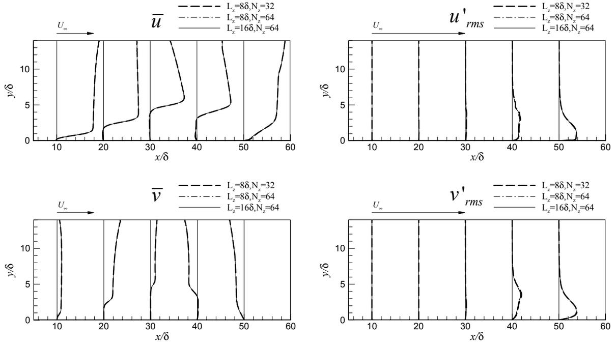
**FIG. A4. Comparisons of the time and spanwise averaged ( $\bar{u}, \bar{v}$ ) and root-mean-squared fluctuation ( $u'_{rms}, v'_{rms}$ ) velocity profiles extracted at the number of streamwise locations for the different spanwise domain sizes and resolutions. The arrow indicates the scale of the inflow freestream velocity.  $L_z$ : spanwise domain size,  $N_z$ : number of grid points in the spanwise direction.**
