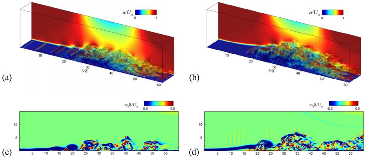
**FIG. 6.** Instantaneous flow fields for the control cases with the ZNMF synthetic jet. 3D vortical structure visualized by the iso-surface of the second invariant of the velocity gradient ( $Q_2$ ) for the sinusoidal (SIN) jet case with  $F_m^+=1$  (a), and the burst modulation (BM) jet with  $F_c^+=10$ ,  $F_m^+=1$ , and DC=50% (b). Spanwise vorticity ( $\omega_z$ ) contours for the SIN jet (c) and the BM jet (d).
