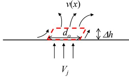
**FIG. A6. A schematic for the control volume (dashed line) near the wall location where the synthetic jet is modeled as the velocity boundary condition. The control volume is taken along the local streamlines.**
