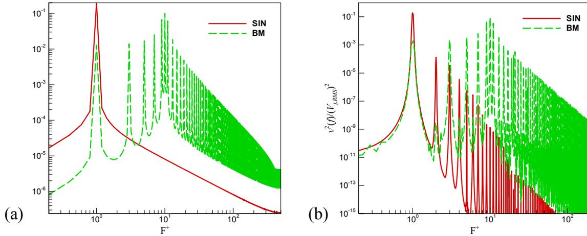
**FIG. 9. (a) Frequency spectra of the synthetic jet velocity input signal. (b) power spectra of vertical velocity monitored on the synthetic jet outlet port in the flow field. The spectral energy is normalized by the RMS of synthetic jet input velocity. SIN: sinusoidal jet at  $F_m^+=1$ , BM: burst modulated jet with  $F_c^+=10$ ,  $F_m^+=1$ , and DC=50%.**
