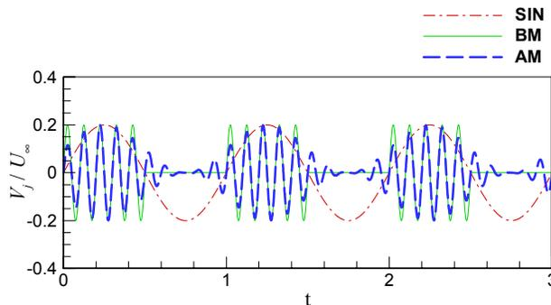
FIG. 1. Synthetic jet profiles. SIN: sinusoidal actuation (Eq. 2), BM: burst modulation with  $f_m=1$ ,  $f_c=10$ ,  $N=10$ , and DC=50% (Eq. 3), AM: sinusoidal amplitude modulation with  $f_m=1$  and  $f_c=10$  (Eq. 4).
