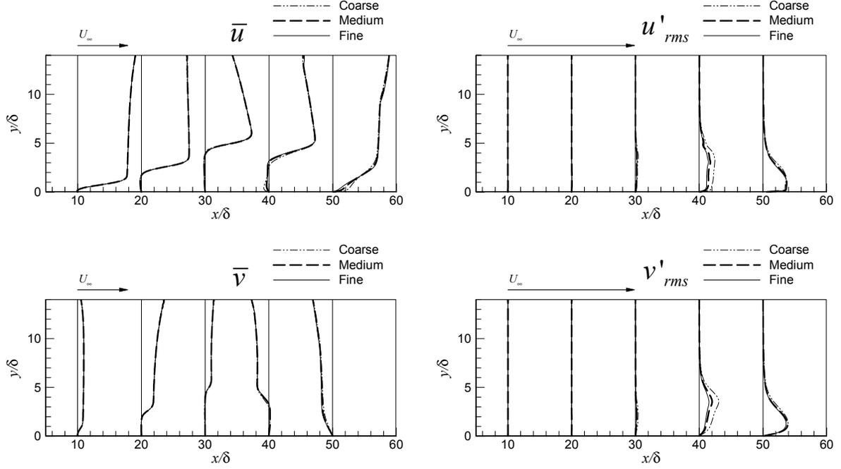
**FIG. A2. Comparisons of the time and spanwise averaged ( $\bar{u}, \bar{v}$ ) and root-mean-squared fluctuation ( $u'_{rms}, v'_{rms}$ ) velocity profiles extracted at the number of streamwise locations for the different grid resolutions. The arrow indicates the scale of the inflow freestream velocity.**
