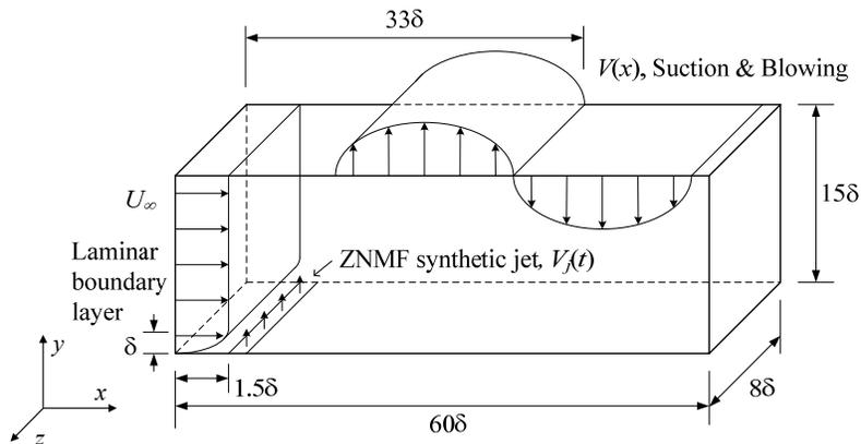
**FIG. 2. Schematic of a simulation set-up.**
