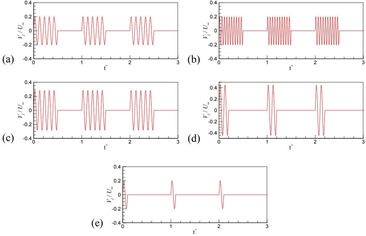
**FIG. 7. Synthetic jet profiles for the burst modulation cases listed in Table 1 (a-e).**
