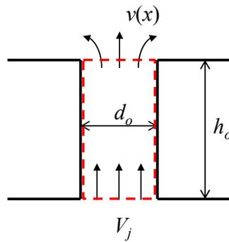
**FIG. A5. A schematic of the synthetic jet outlet slot. Dashed box indicates the control volume for the analysis of pressure drop through the slot.**
