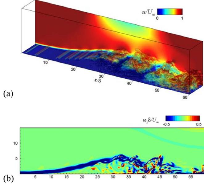
**FIG. 10. Instantaneous flow fields for the sinusoidal jet control at  $F^+=2$ . (a) Vortex structures visualized by the iso-surface of the second invariant of velocity gradients ( $Q_2$ ), (b) Spanwise vorticity ( $\omega_z$ ) contours.**
