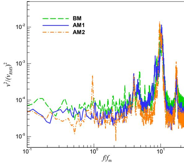
**FIG. 17. Normalized energy spectra of the output jet velocities from the actuator measured in the experiments for the various input energy modulation schemes; BM: burst modulation (Eq. 3) with DC=50%, AM1: amplitude modulation by Eq. 4, and AM2: amplitude modulation by Eq. 9. The modulation frequency is  $f_m$  and the actuator driving frequency is  $f_c=10f_m$ .**
