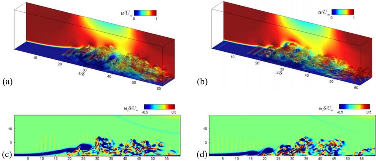
**FIG. 13. Instantaneous flow fields for the control cases with the amplitude modulated synthetic jet. 3D vortical structure visualized by the iso-surface of the second invariant of velocity gradients ( $Q_2$ ) for the AM1 jet (a) and AM2 jet (b) with  $F_c^+=10$ ,  $F_m^+=1$ . Spanwise vorticity ( $\omega_z$ ) contours for the AM1 jet (c) and AM2 jet (d).**
