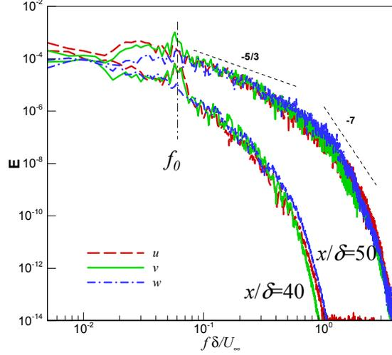
**FIG. 4. Velocity spectra at  $x/\delta=40$  &  $50$ , located  $2\delta$  above from the wall for the baseline case. A discrete peak associated with the vortex shedding in the bubble is observed and is identified as  $f_0$ .**
