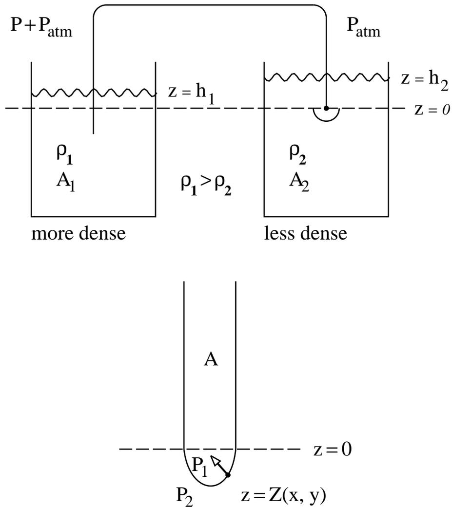
Figure A. Sketch of a Pressure Controlled Drop Experiment.
