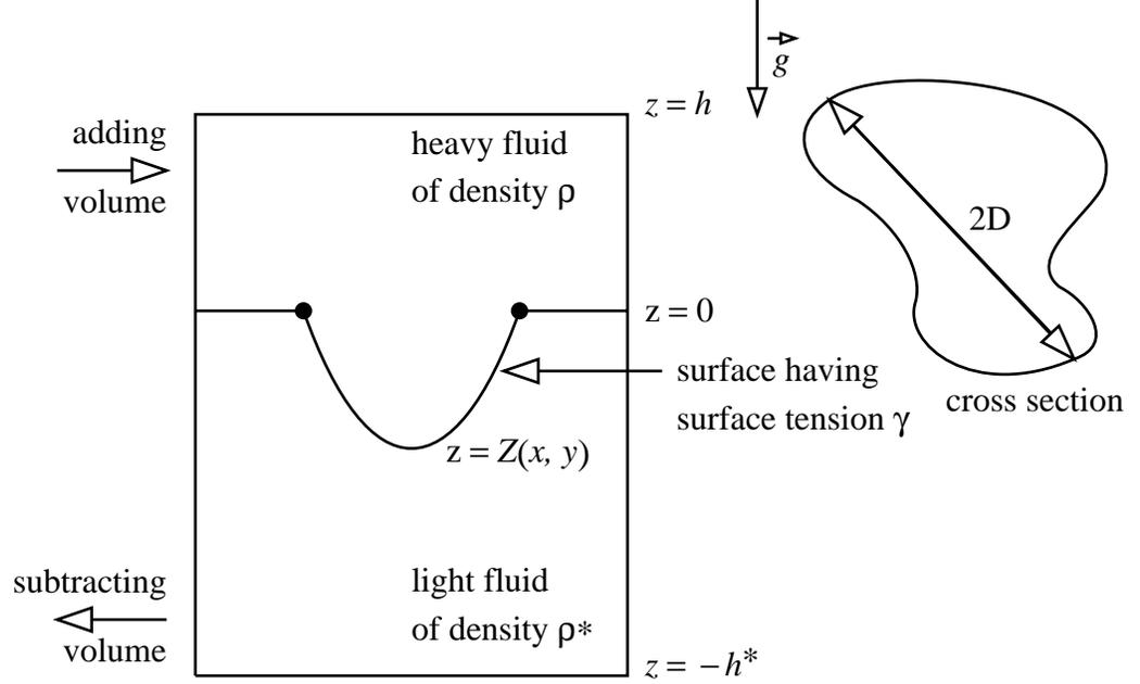
Figure 1. A Sketch of a Drop Pinned Along a curve,  $\mathcal{C}$ , Bounding a Cross Section,  $\mathcal{A}$ , Under Volume Control, Experiment I.
