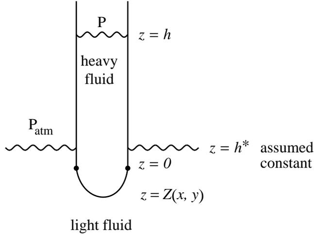
Figure 2. A Sketch of a Drop Under Pressure Control, Experiment II.
