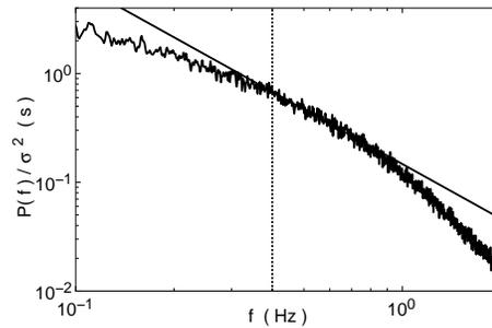
FIG. 5. The normalized temperature power spectrum  $P(f)/\sigma^2$  as a function of the frequency  $f$  in Hz for  $T_b - T_{on} = 10.6$  K and 2-phase flow at the sample center. The solid line is a power-law fit with the exponent fixed at  $-5/3$ . The vertical dotted line indicated an estimate of the lower limit of an inertial range at about 0.4 Hz.
