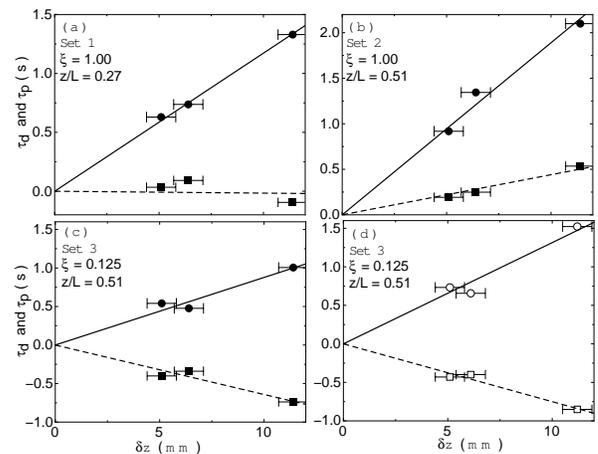
FIG. 7. Plots of  $\tau_p$  (squares) and  $\tau_d$  (circles) as a function of  $\delta z$ . (a), (b), and (c) are for 2-phase flow and  $T_b - T_{on} = 7.82$  K (run 1511203). (d) is for 1-phase flow and  $T_b - T_{on} = 8.45$  K (run 1512075). The data yield (a):  $\alpha_p = -0.002$ ,  $\alpha_0 = 0.117$  s/mm; (b):  $\alpha_p = 0.044$ ,  $\alpha_0 = 0.189$  s/mm; (c):  $\alpha_p = -0.064$ ,  $\alpha_0 = 0.088$  s/mm; (d):  $\alpha_p = -0.075$ ,  $\alpha_0 = 0.131$  s/mm.
