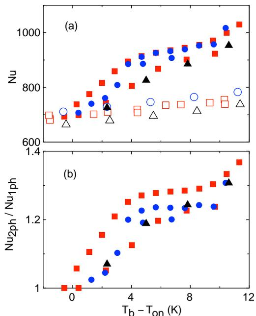
FIG. 9. (a) The Nusselt number for 1-phase flow ( $Nu_{1ph}$ , open symbols) and 2-phase flow ( $Nu_{2ph}$ , solid symbols) and (b) the ratio  $Nu_{2ph}/Nu_{1ph}$  as a function of the superheat  $T_b - T_{on}$ . Circles (blue): Cell A. Triangle: Cell B. Squares (red): NG [29].
