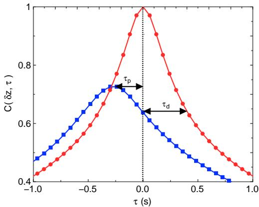
FIG. 4. The auto-correlation function (circles, red) and cross-correlation function (squares, blue) for  $T_b - T_{on} = 10.6$  K and 2-phase flow of thermistors V1-5 and V1-6 ( $\delta z = 6.4$  mm, see Tables I and II). The auto-correlation function is the average of those at the two locations. The time intervals  $\tau_p = -0.266$  s and  $\tau_d = 0.407$  s are illustrated by the arrows.
