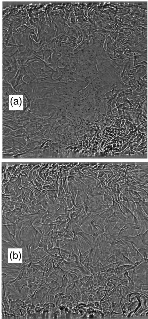
FIG. 10. Shadowgraph images taken from the side for (a) 2-phase and (b) 1-phase flow (from NG [30]). They show a horizontal average over the entire width of the sample. The tiny dark dots in (a) (hardly visible) rising through the center are the bubbles. The corresponding movies in the supplementary material of Ref. [30] reveal a more detailed picture of the flow dynamics.
