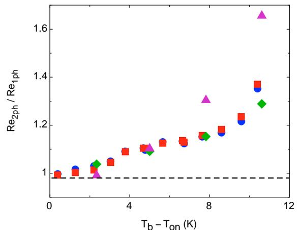
FIG. 19. The relative increase of Reynolds numbers in 2-phase flow compared to 1-phase flow as a function of the superheat. Circles (blue):  $Re_{ac}$ . Diamonds (green):  $Re_{f_0}$ . Squares (red):  $Re_{sl}$ . Triangles (purple):  $Re_V$  for  $\bar{z}/L = 0.25$ ,  $\xi = 1.00$  from Fig. 14.
