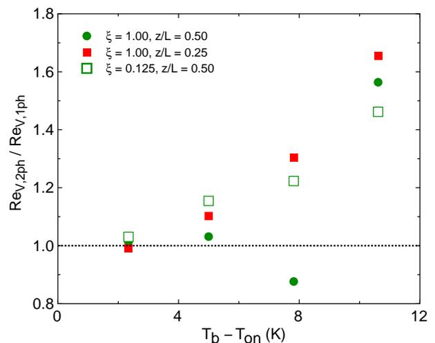
FIG. 14. The ratio  $Re_{V,2ph}/Re_{V,1ph}$  as a function of the superheat  $T_b - T_{on}$ .
