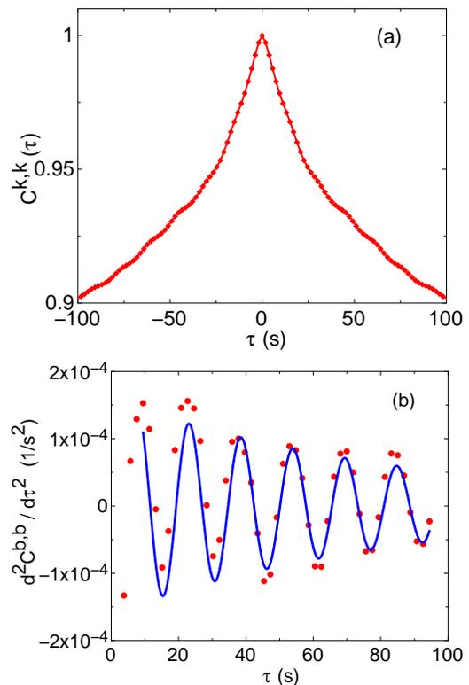
FIG. 15. (a): Azimuthally averaged auto-correlation function for the largest superheat  $T_b - T_{on} = 10.4$  K and 2-phase flow in cell A for  $k = b$ . (b): Points: The second derivative of the averaged auto-correlation function for  $k = b$  in (a) with respect to  $\tau$ . Line: Fit of Eq. 23 to the data.
