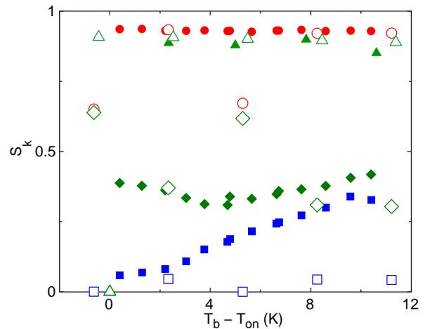
FIG. 12. The parameter  $S_k$  (Eq. 20) describing the strength of the LSF. Circles (red), diamonds (green), and squares (blue) correspond to the lower ( $k = b$ ), middle ( $k = m$ ), and upper ( $k = t$ ) set of thermistors in cell A respectively. The triangles (green) are for  $k = m$  of cell B. Open symbols: 1-phase flow. Solid symbols: 2-phase flow.
