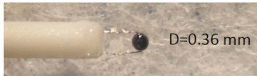
FIG. 3. Photograph of a type 111-104HAK-H01 (0.36 mm diameter) thermistor mounted through its 0.9 mm diameter ceramic rod. Adapted from Fig. 2 of Ref. [21].
