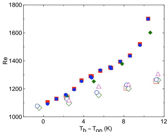
FIG. 16. Reynolds numbers as a function of the superheat  $T_b - T_{on}$ . Circles (blue):  $Re_{ac}$  at the lower plane  $k = b$  of cell A. Squares (red):  $Re_{sl}$  based on the sloshing-mode oscillations at the lower plane  $k = b$  of cell A. Diamonds (green):  $Re_{f_0}$  from temperature oscillations in the interior of cell B. Triangles (purple):  $Re_U$  for  $\xi = 0.125$ ,  $\bar{z}/L = 0.50$  from Fig. 13 (c). Open symbols: 1-phase flow. Solid symbols: 2-phase flow.
