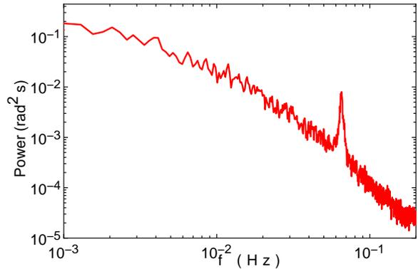
FIG. 17. The power-spectral density of the displacement angle  $\theta'$  at the lower plane  $k = b$  in cell A for 2-phase flow at a superheat  $T_b - T_{on} = 10.4$  K.
