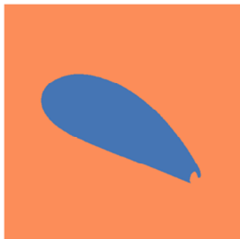
(d) Shape of the secondary lobe under coarse grid (700 points across the initial void diameter)
