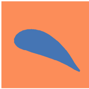
(a) Shape of the secondary lobe under coarse grid (100 points across the initial void diameter)
