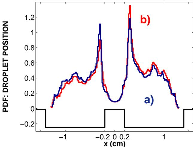
FIG. 11. Histograms of droplet position. Here,  $\Gamma = 4.5$ ,  $\Gamma_F \approx 5$ ,  $L = 1.2\text{cm}$ ,  $L_b = 0.40\text{cm}$  and depth  $h_b = 0.092\text{cm}$ . **a)** PDF for a single simulation with  $t \in [0, 30000T_F]$ . **b)** PDF for only 6 simulations with different initial droplet positions (3 in each cavity) and  $t \in [0, 5000T_F]$ .
