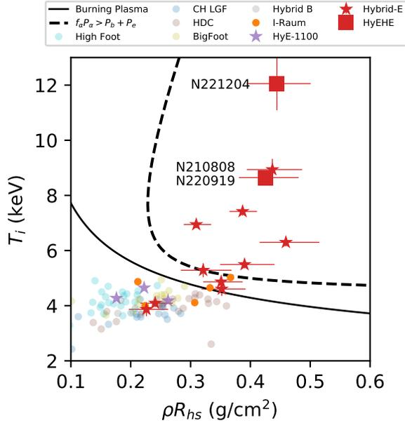
FIG. 7. Hot-spot ion temperature and areal density. Thresholds for the burning-plasma criteria (solid line) and static self-heating (dashed line) are shown with NIF data. Here the ion temperature is inferred from the width of the DD neutron spectra.
