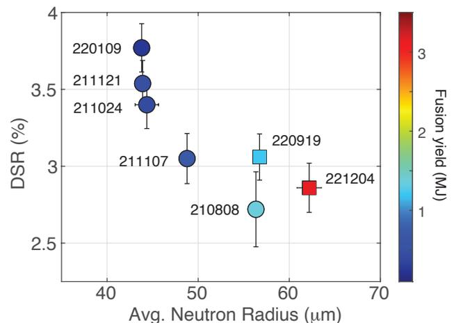
FIG. 4. The  $4\pi$  averaged down scattered ratio (DSR) vs. the average radius of neutron emission for the 1.9 MJ design (circles) and 2.05 MJ design (squares). The color of the datum correspond to the fusion yield of the experiment.
