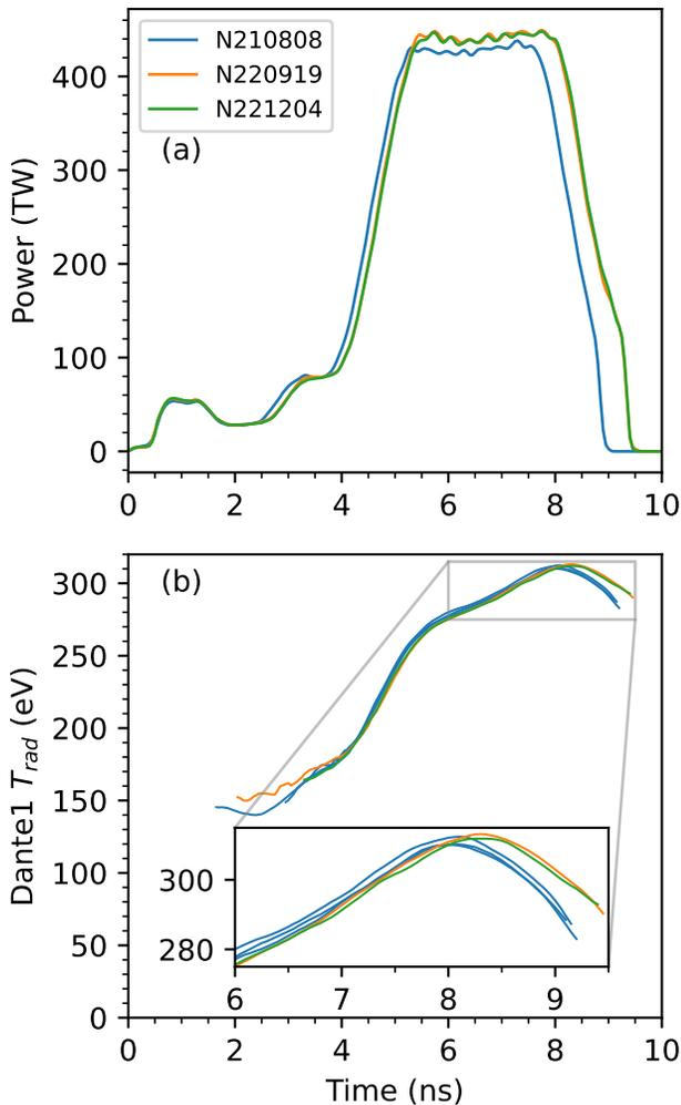
FIG. 1. Top (a): Laser pulses as delivered for N220919 and N221204 versus N210808. Bottom (b): Measured radiation temperature ( $T_{rad}$ ) from Dante 1 versus time. Since the Dante 1 data are not available for N210808, data from several shots that repeated the same laser pulse are shown in blue. Dante data are shown until 100ps before peak nuclear production.
