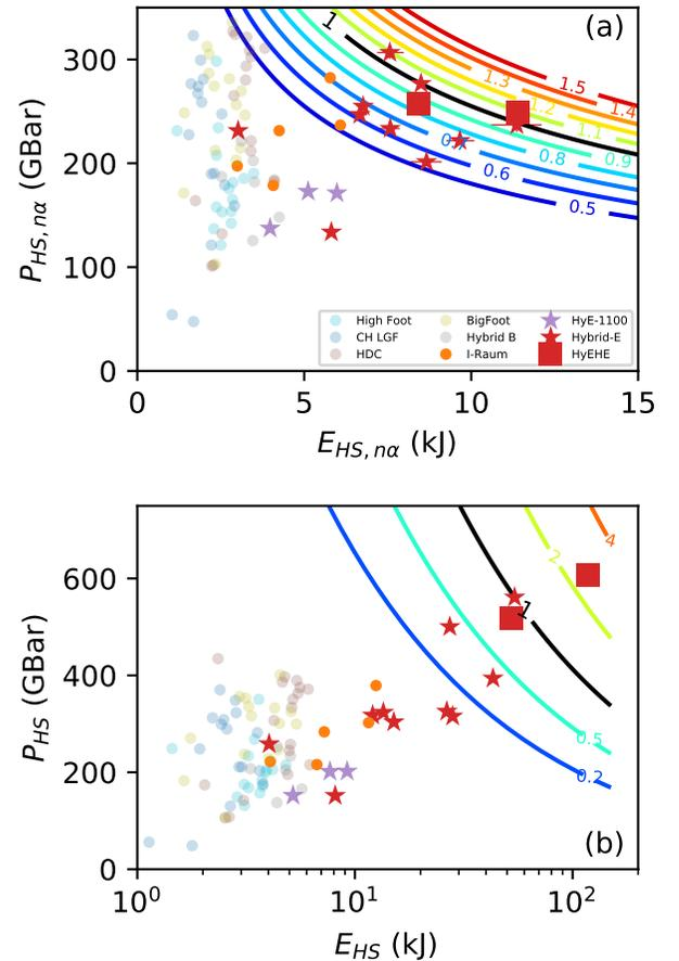
FIG. 9. Inferred hot-spot pressure and energy, inferred without the presence of self-heating (top, a) and directly for the burn-on experiments (bottom, b). Contours of  $EP^2$  relative to N210808 in both cases are shown.
