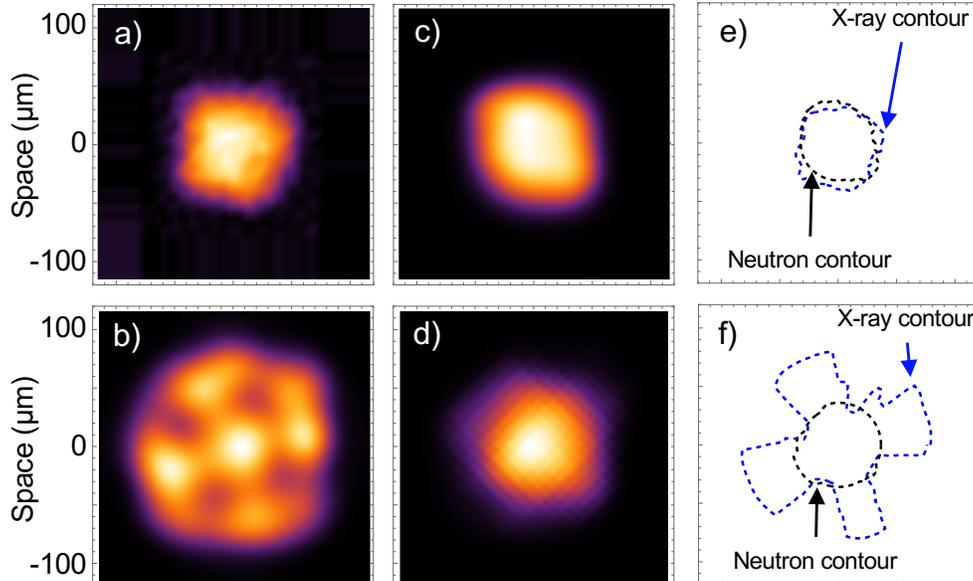
FIG. 6. X-ray and neutron emission measurements from N210808 (top row) and N221204 (bottom row). Time integrated x-ray emission ( $> 10$  keV) from N210808, a), and from N221204, b). Time integrated neutron emission from N210808 c) and from N221204, d). Comparison of contours that enclosed 50% of the x-ray and neutron emission for N210808 e), and for N221204, f). Further details of the x-ray imaging diagnostic are given in the appendix.
