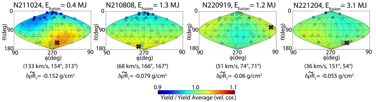
FIG. 2. Angularly resolved nuclear activation maps from a series of experiments showing a progression of reduced mode 1 symmetry impact. Shown below each subplot are the hot spot velocity and maximum difference in  $\rho R$  inferred from the variation in nuclear activation. On the figures, X marks the direction of the hot spot velocity, with the red ellipse denoting the uncertainty and the circles = Real Time Nuclear Activation Diagnostic (RT-NAD) locations.
