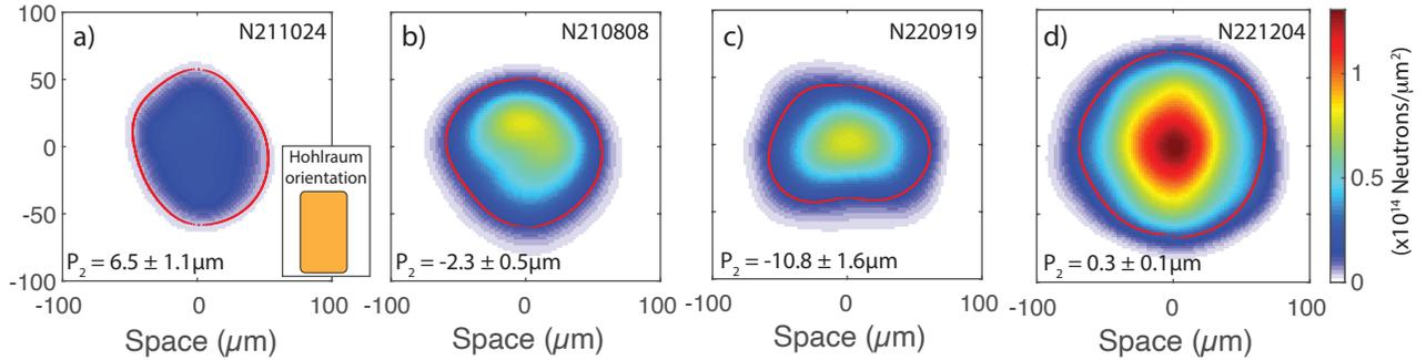
FIG. 3. Equatorial view of the time integrated neutron emission showing the impact of low mode asymmetries on the fusion yield for pairs of experiments conducted with 1.9 MJ of laser energy a-b) and 2.05 MJ of laser energy c-d). The 17% contour of emission is denoted by the solid red line. The inset in a) shows the hohlraum orientation with respect to the image and for each experiment the mode 2 amplitude,  $P_2$  is given. The mode 1 amplitude for each experiment is given in Fig. 2
