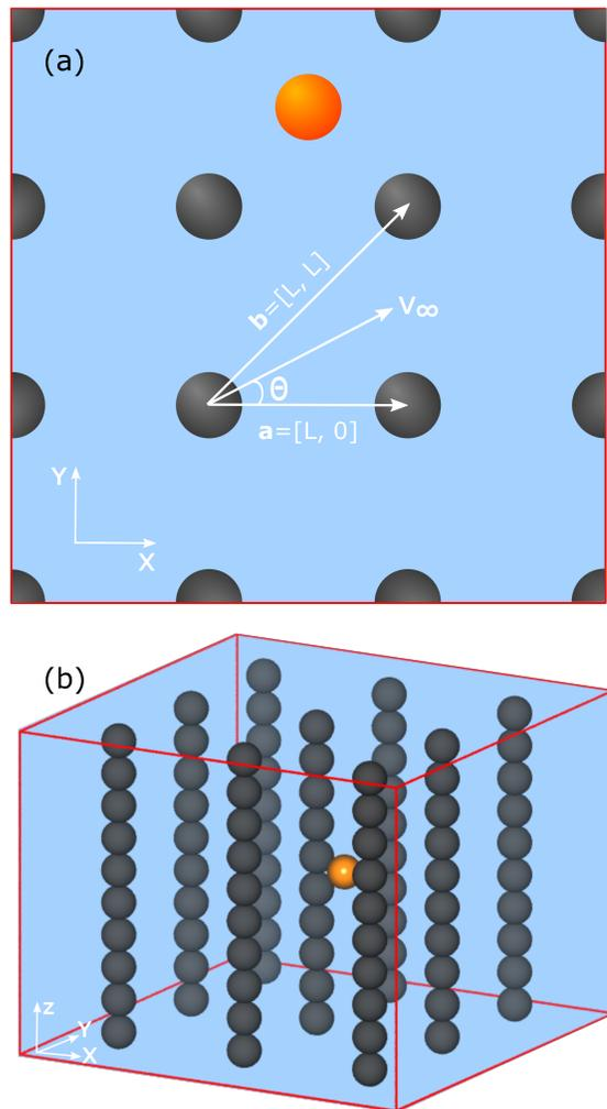
FIG. 1. (a) Two-dimensional orthographic projection of a square nanopost array in the  $x - y$  plane of the simulation cell. (b) Three-dimensional perspective view of a section of a square nanopost array. The spheres representing the nanoposts (grey, np) and the diffusing particle (orange, p) have the same diameter (i.e.,  $d_{np} = d_p$ ).
