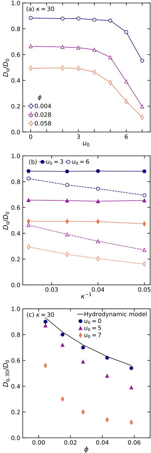
FIG. 3. Normalized in-plane diffusion coefficients  $D_q/D_0$  as functions of (a) potential strength  $u_0$  for  $\kappa = 30$  and (b) potential range  $\kappa^{-1}$  for  $u_0 = 3$  and  $6$ . (c) Comparison of normalized three-dimensional diffusion coefficients  $D_{q,3D}/D_0$  as functions of nanopost volume fraction  $\phi$  with a hydrodynamic model for hindered diffusion [49]. Estimated uncertainties are smaller than the symbol sizes.
