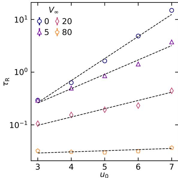
FIG. 6. Characteristic trapping time  $\tau_R$  as a function of the magnitude of the potential strength  $u_0$  for  $\kappa = 30$  at different  $V_\infty$ . The black dashed lines show fits to the function  $\tau_R = c_1 \exp^{-c_2 u_0 / k_B T}$ , where  $c_1$  and  $c_2$  are fitting constants.
