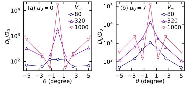
FIG. 10. Normalized longitudinal dispersion coefficient  $D_L/D_0$  as a function of flow orientation  $\theta$  in a square array with  $\phi = 0.058$  for attractive potentials with  $\kappa = 30$  and (a)  $u_0 = 0$  and (b)  $u_0 = 6$ .
