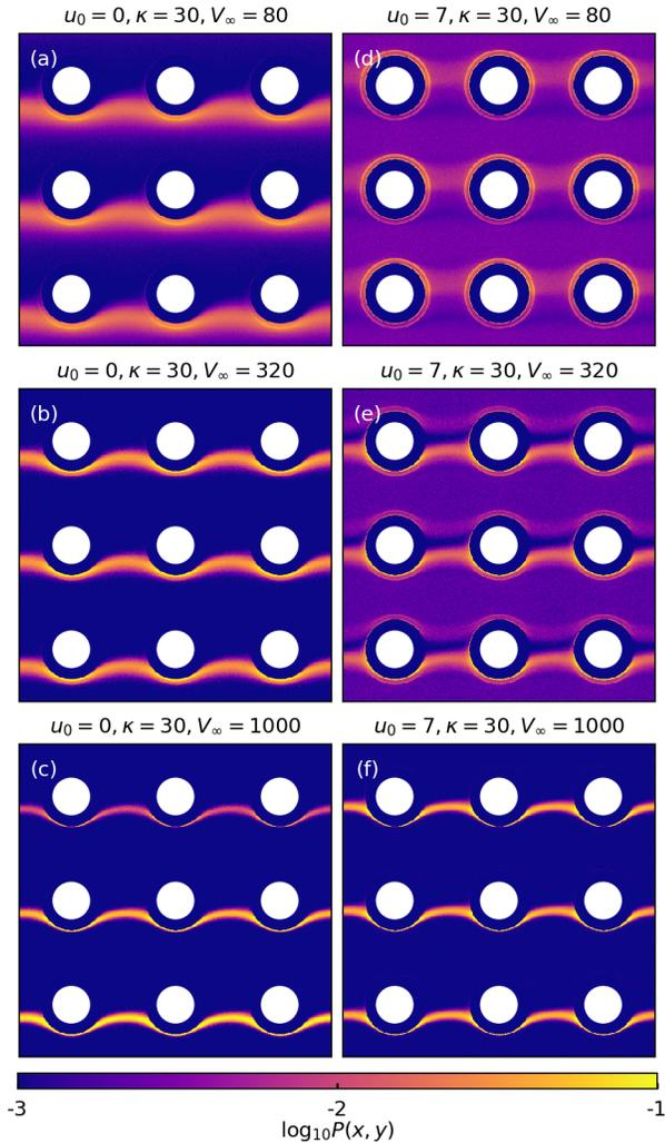
FIG. 9. Log-probability density distributions of particle positions  $\log_{10} P(x, y)$  for  $u_0 = 0$  (a,b,c) and  $u_0 = 7$  (d,e,f) at  $V_\infty$  (a,b) 80, (c,d) 320, and (e,f) 1000 for flow orientation  $\theta = 1.25^\circ$ . The intense blue color corresponds to regions where  $\log_{10} P(x, y) < -3$ .
