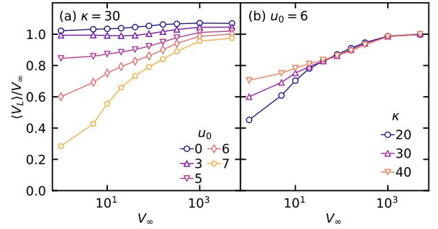
FIG. 4. Normalized average particle velocities  $\langle V_L \rangle / V_\infty$  as functions of uniform suspension velocity  $V_\infty$  at flow orientation  $\theta = 45^\circ$  for (a) different  $u_0$  and fixed  $\kappa = 30$  and (b) different  $\kappa$  and fixed  $u_0 = 6$ . Estimated uncertainties are smaller than the symbol sizes.
