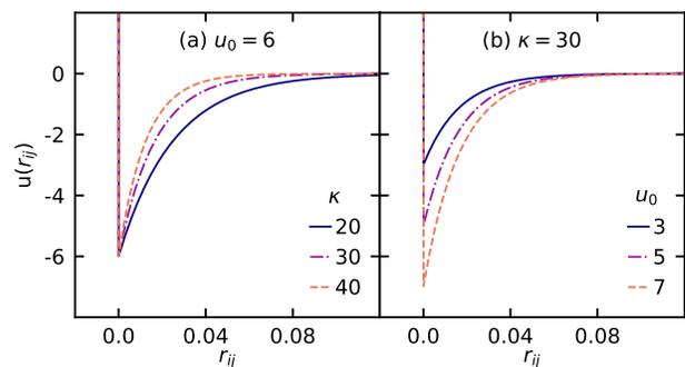
FIG. 2. Yukawa potential with repulsive core  $u(r_{ij})$  (Eq. 1) as a function of the surface-to-surface distance  $r_{ij}$  for (a) different  $u_0$  and fixed  $\kappa = 30$  and (b) different  $\kappa$  and fixed  $u_0 = 6$ .
