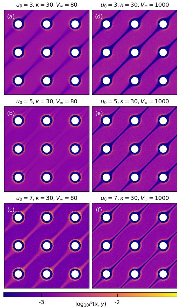
FIG. 7. Log-probability density distributions of particle positions  $\log_{10} P(x, y)$  for  $u_0 = 3$  (a,d), 5 (b,e) and 7 (c,f) at  $V_\infty$  of (a,b,c) 80 and (d,e,f) 1000 for flow orientation  $\theta = 45^\circ$ . The intense blue color corresponds to regions where  $\log_{10} P(x, y) < -3$ .
