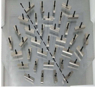
Figure 4: One of the equilibrium configurations of rare-earth magnets in a triangular lattice.
