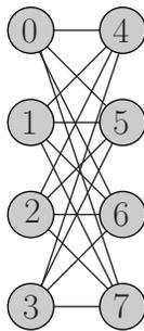
FIG. 6. Cell of chimera graph in D-Wave systems.
