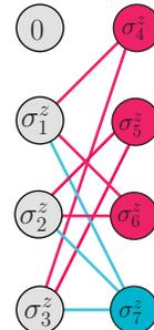
FIG. 7. Three body interactions implemented on the chimera topology.
