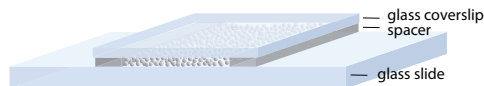
FIG. 2. Diagram of a sample chamber containing a disordered packing of colloidal spheres. The sample chamber consists of a glass slide on the bottom, a glass coverslip on top, and Mylar spacers to set the thickness. It is sealed with UV-curable epoxy.
