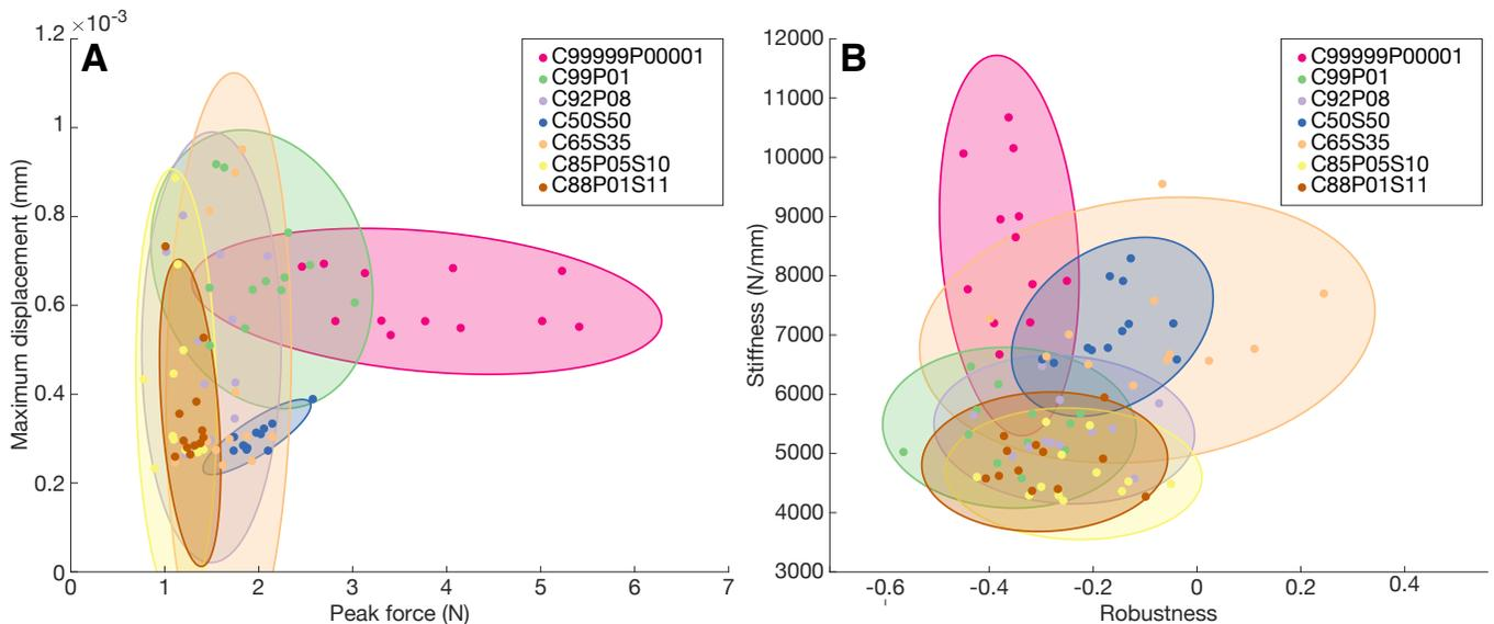
FIG. 4. Ashby plots comparing properties of different optimization parameter sets. Panel A compares the maximum displacement before complete failure with the peak reaction force attained. Panel B compares stiffness, the slope of the force-displacement curve in the linear regime prior to failure, with robustness, measured as the relative change between the peak forces of the original and perturbed models. Shaded ellipses represent  $2\sigma$  confidence intervals.
