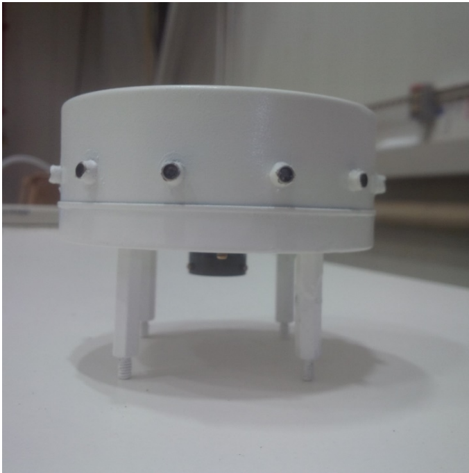
FIG. 1: Photograph of ATSA sun sensor, employing 12 MEPhI-mark Silicon Photomultipliers (SiPM) arranged azimuthally.
