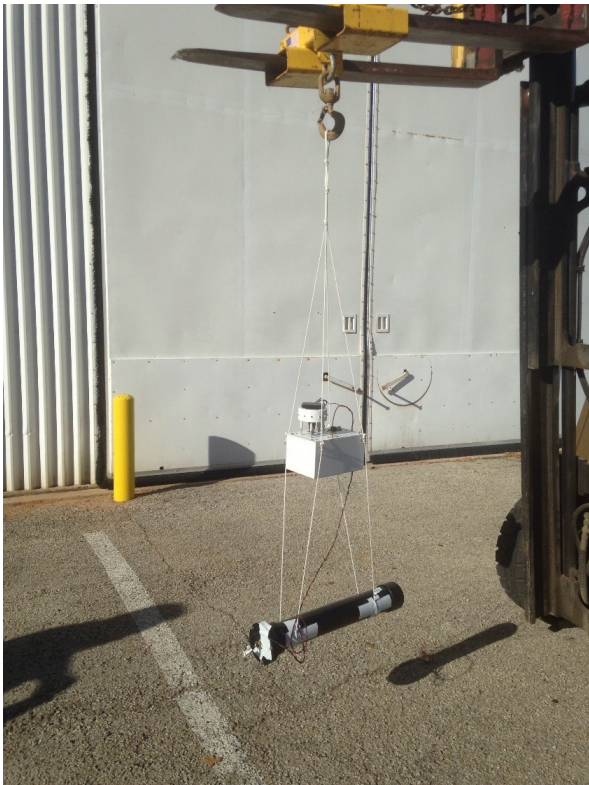
FIG. 5: Photo of HiCal payload taken during pre-flight hang test (June, 2016, Palestine, TX). Motor to drive piezo signal generator and transmitter antenna are enclosed within cylindrical pressure vessel, suspended from CSBF MIP electronics box. Pressure vessel was later painted white prior to flight.
