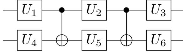
Figure 3: Decomposition of FF-gate for IBM quantum computer.
