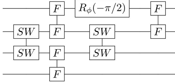
Figure 1: Quantum circuit for preparing the measurement in the momentum space. We simplified the inverse quantum Fourier transform. This circuit maps the momentum states  $|+k\rangle$  and  $|-k\rangle$  into the  $|0100\rangle|0100\rangle$  and  $|1000\rangle|1000\rangle$  computational basis states, respectively. The entangling operations were transpiled using CNOTs as entanglers.
