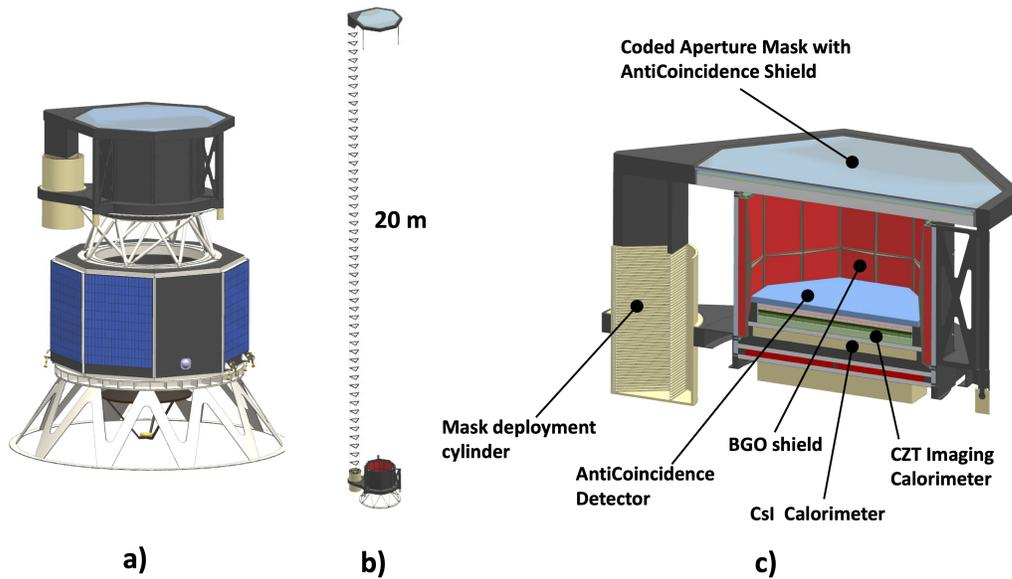
Figure 1: GECCO design concept: a) with mask in stowed position and notional spacecraft bus; b) with mask in deployed position; c) cutaway. [13]
