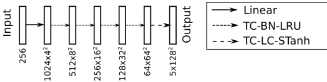
Figure 2: Shown is a diagram of the DCWGAN-GP generator model described in Section III A and indicated in the schematic of Figure 1 as Training Step 1. The input to this generator is a latent-vector consisting of 256 random numbers drawn from a Gaussian distribution with mean equal to zero and variance equal to one ( \mu = 0, \sigma = 1 ). The output is one set of 1^\circ \times 1^\circ maps consisting of the five foreground components. The direction of data flow is indicated by arrows. A solid arrow is a fully connected Linear layer. A short-dashed arrow, labeled TC-BN-LRU, represents a sequence of 1) a 4 \times 4 two-dimensional transposed convolution, 2) a batch normalization, and 3) a leaky rectified linear unit activation function with \alpha = 0.2 . Lastly, a long-dashed arrow, labeled TC-LC-STanh, is a sequence of 1) a 4 \times 4 two-dimensional transposed convolution, 2) a Linear Channel, and 3) a Scaled Tanh activation function. The Linear Channel and Scaled Tanh are defined in Section III A. Note that a transposed convolution upsamples an image by a factor of two.
