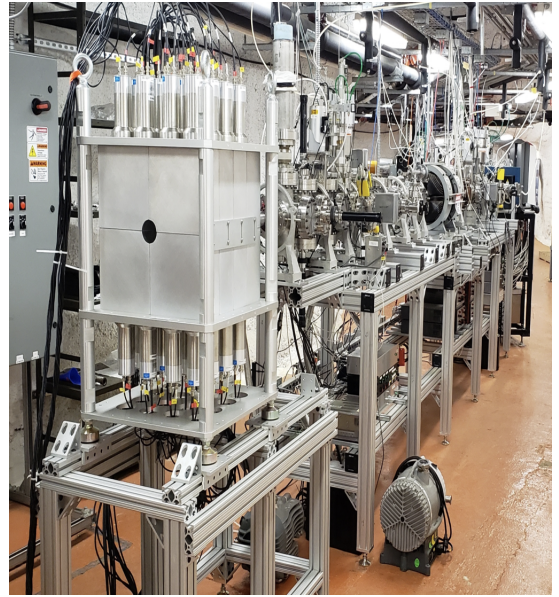
FIG. 3. Experimental setup showing HECTOR placed at the end of the beamline at the CASPAR underground lab. The target was placed at the center of the detector cube.
