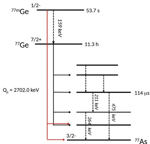
FIG. 6. The decay scheme of  $^{77}\text{Ge}$  and  $^{77m}\text{Ge}$  (red) to  $^{77}\text{As}$  [42, 43]. Events from the  $^{77}/^{77m}\text{Ge}$ -decay are expected to be the dominant contribution induced by cosmogenics to the background in the  $0\nu\beta\beta$ -ROI.
