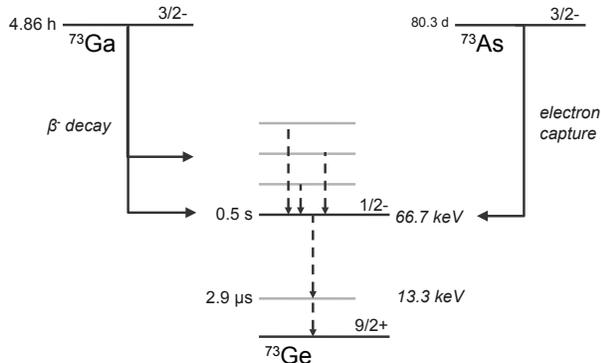
FIG. 3. The decay scheme of  $^{73}\text{Ga}$ ,  $^{73m}\text{Ge}$ , and  $^{73}\text{As}$  to  $^{73}\text{Ge}$  [42, 43].
