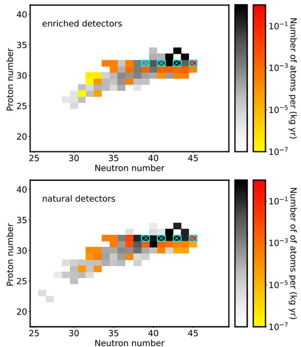
FIG. 1. (Color online) Production rate of isotopes from in-situ cosmogenics and their products with natural detectors (top) and enriched (87%  $^{76}\text{Ge}$ ) detectors (bottom) at the 4850-ft level. The colored scale represents isotopes with the potential to contribute background for  $0\nu\beta\beta$  while the grey-scale isotopes do not contribute to the region of interest (ROI). The germanium isotopes with odd neutron number analyzed in this paper are outlined in cyan.
