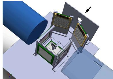
FIG. 1. Experimental setup for the  $\beta$  decay of  $^{20}\text{Na}$ . The simultaneous measurement of  $\beta$ ,  $\alpha$  and  $\gamma$  transitions from the  $^{20}\text{Na}$  decay is realized by using five pieces of MSQ, two pieces of DSSD and two HPGe detectors, respectively. The top MSQ is removed to show the collection foil.
