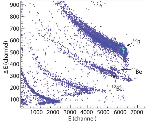
FIG. 1. The  $\Delta E - E$  spectrum obtained using one of the recoil detector telescopes with  $^{12}\text{B}$  incident on the  $(\text{CD}_2)_n$  target. The data shown required a coincidence with a particle in the PSD array. The particle groups labeled  $^{11}\text{Be}$  ( $^{10}\text{Be}$ ) and  $^{12}\text{B}$  are from neutron bound (unbound) states in  $^{11}\text{Be}$  and the elastic scattering of  $^{12}\text{B}$ , respectively.
