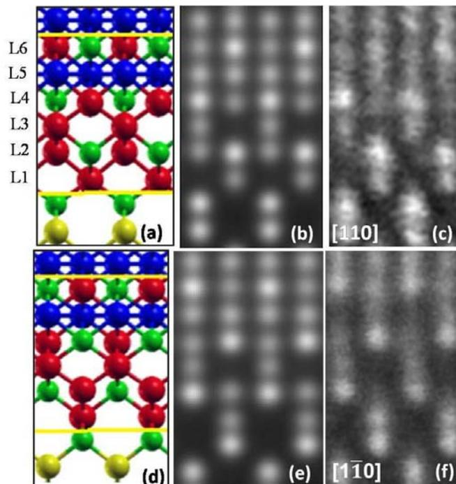
**Figure 7:** (Color online); (a) and (d) Ball-and-stick representation of the DFT-relaxed interface structure for the Co-initiated model along the  $[110]$  and  $[1\bar{1}0]$  directions, and (b) and (e) corresponding frozen-phonon multi-slice STEM simulations image. (c) and (f) High-resolution Z-contrast STEM images of the CMS/GaAs interface (Co-initiated sample). Color scheme: Co – blue, Mn – red, As – green, and Ga – yellow.
