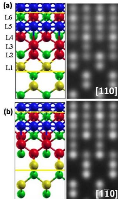
**Figure 6:** (Color online); Ball-and-stick representation of the DFT-relaxed interface structure for the MnSi-initiated interface without Si at L3 along the [110] (a) and  $[1\bar{1}0]$  (b) directions (left images), and corresponding frozen-phonon multislice STEM simulations image (right images), Color scheme: Co – blue, Mn – red, As – green, and Ga – yellow.
