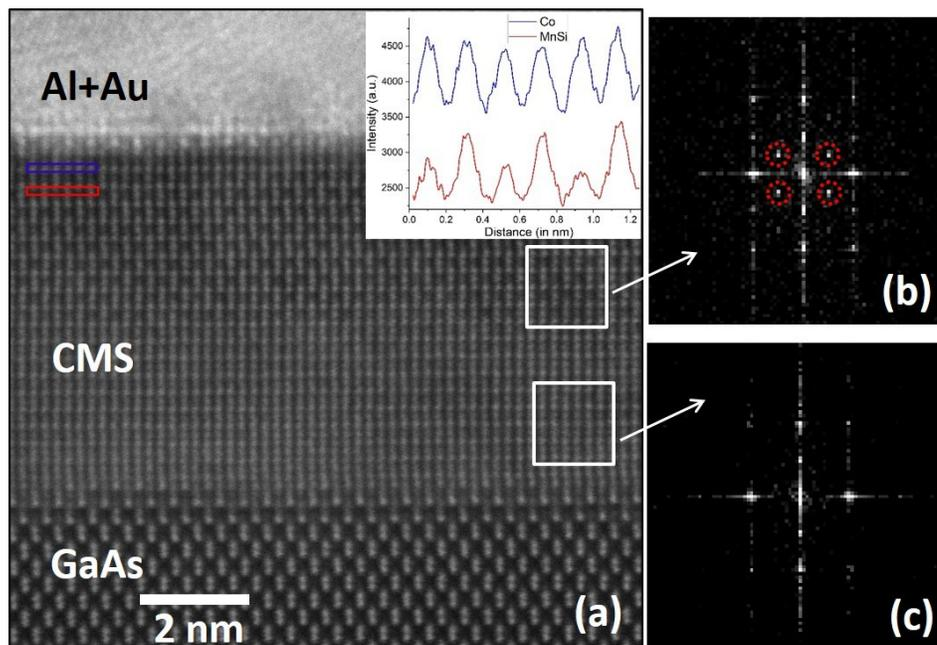
**Figure 1:** (Color online); (a) Cross-sectional high-resolution HAADF-STEM image of CMS film on GaAs(001) surface taken along the  $[1\bar{1}0]$  zone axis of a GaAs substrate and the line profile of Co and MnSi (inset figures), (b) and (c) shows the FFT of the region mentioned in (a) which indicates the  $L2_1$  and  $B_2$  phase respectively.
