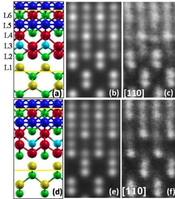
**Figure 5:** (Color online); (a) and (d) Ball-and-stick representation of the DFT-relaxed interface structure for the MnSi initiated model with Si at L3 along the  $[110]$  and  $[1\bar{1}0]$  directions, and (b) and (e) corresponding frozen-phonon multislice STEM simulations image. (c) and (f) High-resolution Z-contrast STEM images of the CMS/GaAs interface (MnSi initiated sample). Color scheme: Co – blue, Mn – red, Si – turquoise, As – green, and Ga – yellow.
