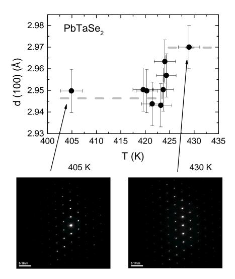
FIG. 11: In-plane TEM results at elevated temperatures. Upper panel: the basal plane d-spacing, d(100) as a function of temperature. Lower panels: selected area diffraction patterns at 405 K and 430 K. Gray dashed line is a guide to the eye.
