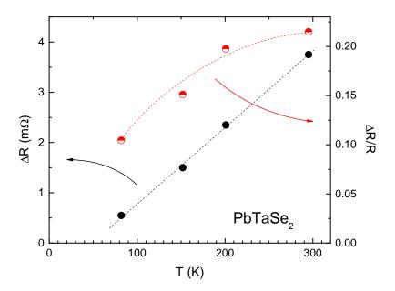
FIG. 7: (Color online) Temperature-dependent absolute and relative (to the average resistance below and above the transition) resistance jump at the apparent structural transition. Dashed lines are the guides for the eye.
