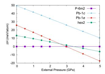
FIG. 17: (Color online) Formation enthalpy differences of the PbTaSe<sub>2</sub> structures under pressure with respect to the  $P\bar{6}m2$  structure.
