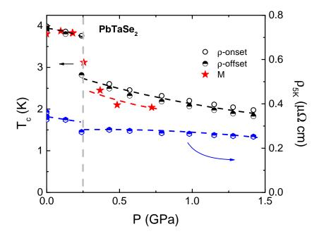
FIG. 3: (Color online)  $T_c$  as determined from resistivity and magnetization measurements (left Y-axis), and normal state resistivity at 5 K (right Y-axis) as a function of pressure. Dashed vertical line shows P = 0.25 GPa location. Dashed lines through the experimental points are guides for the eye.
