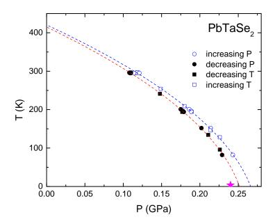
FIG. 9: (Color online) Pressure dependence of the apparent structural transition. Open symbols are points obtained on increase of pressure or temperature, filled symbols - on decrease. Dashed lines are from the second order polynomial fits of the P(T) data. Star - data point corresponding to two-step superconducting transition in Fig. 2a.
