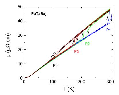
FIG. 5: (Color online) Temperature-dependent resistivity measured on warming and on cooling at four different, small pressures in the piston-cylinder cell, 0.05 GPa  $< P_1 < P_2 < P_3 < P_4 < 0.39$  GPa (see text for more details).
