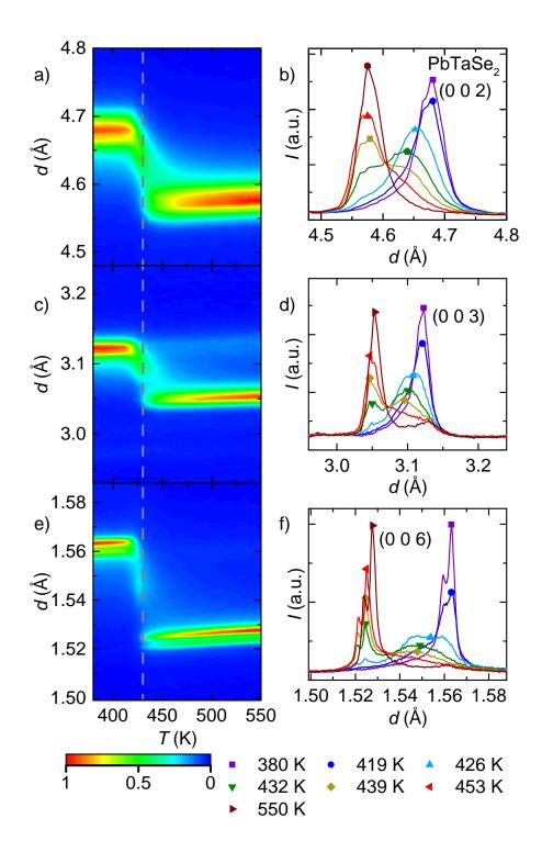
FIG. 10: (Color online) Evolution of the peaks corresponding to  $(0\ 0\ 2)$ ,  $(0\ 0\ 3)$ , and  $(0\ 0\ 6)$  reflections at elevated temperatures (measured on heating) plotted as color maps of d-spacing vs. temperature [a), c), e)] (different colors correspond to different normalized intensities, the color scale is presented in the bottom left part of the figure), and selected  $2\theta$  scans plotted as intensity vs. d-spacing at different temperatures [b), d), f)].
