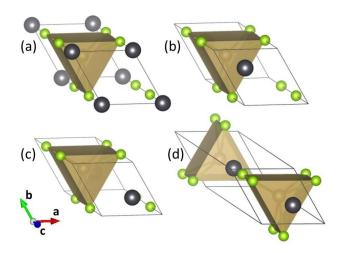
FIG. 15: (Color online) Crystal structures of (a)  $P\bar{6}m2$ , (b) Pb-1c, (c) Pb-1e and (d) hex2 PbTaSe<sub>2</sub> structures. Dark grey and green balls are Pb and Se atoms. Shaded balls at centers of brown triangle prisms are Ta atoms.
