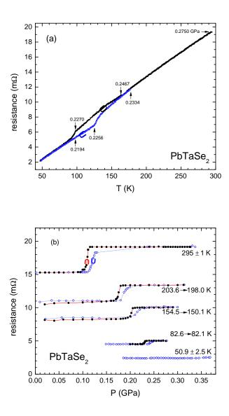
FIG. 6: (Color online) Examples (a) of temperature sweeps at almost constant, continuously monitored, gas pressure, and (b) of pressure sweeps close to constant temperature. Numbers in panel (a) indicate measured pressure in GPa, in panel (b) change of temperature during the run. Arrows on the curves indicate the direction of the temperature/pressure changes: open symbols: increase, filled symbols - decrease.
