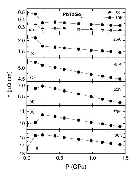
FIG. 8: Zero field, normal state resistivities of the PbTaSe<sub>2</sub> at selected temperatures plotted as a function of pressure. The plot is assembled based on measurements in a piston cylinder cell. Data for T = 5 K are the same as plotted in Fig. 3.
