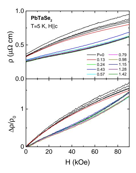
FIG. 4: (Color online) Low temperature, T=5 K, field dependent magnetoresistance at different pressures (listed in the upper panel in units of GPa), plotted as  $\rho(H)$  and  $\Delta\rho/\rho_0(H)$ . Note: for both panels the four P = 0 data sets, as well as the P=0.13 GPa data set form an upper manifold, and the  $P \geq 0.24$  GPa data sets form a lower manifold.
