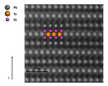
FIG. 12: (Color online) Atomic resolution TEM imaging at room temperature. The arrow shows c-direction. Note fairly large gap between the Ta/Se layer and Pb layer.
