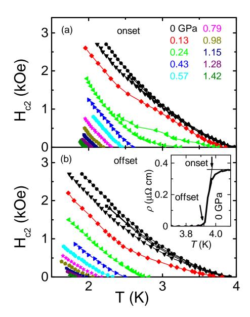
FIG. 19: (Color online)  $H_{c2}(T)$  data for H|c obtained from resistivity (onset and offset criteria) at different pressures. Inset shows the definition of the criteria used. Note that there are two sets of data for P = 0.24 GPa using the onset criterion. Since the resistively measured superconducting transition at this pressure has two steps [Fig. 2(a)] and this shape of the transition persists in applied magnetic fields, two possible onset criteria were used.
