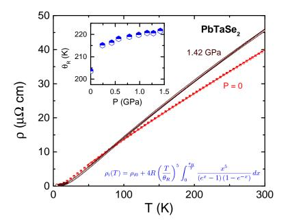
FIG. 14: (Color online) Examples of the Bloch - Grüneisen fits of resistivity, using the equation in the bottom of the plot<sup>36</sup>. Fits of the data between 50 K and 300 K are shown as lines for P = 0 and P = 1.42 GPa. Inset: Debye temperature as a function of the low temperature pressure values (see text for more details).
