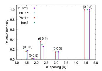
FIG. 16: (Color online) Simulated XRD patterns of four different PbTaSe<sub>2</sub> structures considered in first principles calculations. The peak indexes of the *hex2* structure are (0 0 2l) of the labeled ones and the diffraction intensities of all structures are normalized by the intensity of their (0 0 2)-peak. (See text and Fig. 15 for details.)
