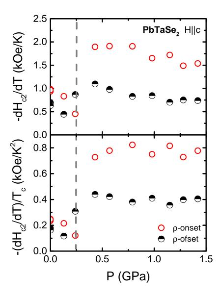
FIG. 20: (Color online) Pressure dependence of the initial, close to  $T_c(H=0)$ , slope of the upper critical field for H||c, plotted as  $-dH_{c2}/dT(P)$  and  $-(dH_{c2}/dT)/T_c(P)$
