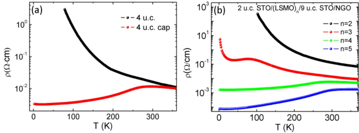
**Fig. 5**  $T$ -dependence of the resistivity for (a) 4 u.c. LSMO grown on a 9 u.c. STO buffered NGO (110) substrate with and without 2 u.c. STO capping; and (b) the different thickness of LSMO films grown on a 9 u.c. STO buffered NGO (110) substrate and capped with 2 u.c. STO capping layer.
