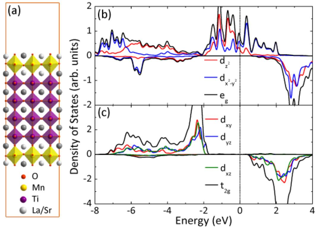
**Figure 4.** (a) The optimized slab model of a single u.c. thickness of LSMO film on STO(001) for the DFT+U ( $U_{\text{Mn}} = 2.0$  eV and  $U_{\text{Ti}} = 8.0$  eV) calculations. The calculated orbital- and spin-resolved densities of states for both (b)  $e_g$  and (c)  $t_{2g}$  orbitals. The single layer LSMO film with ferromagnetic order is subjected to a tensile strain with in-plane lattice constant of  $3.905 \text{ \AA}$ .
