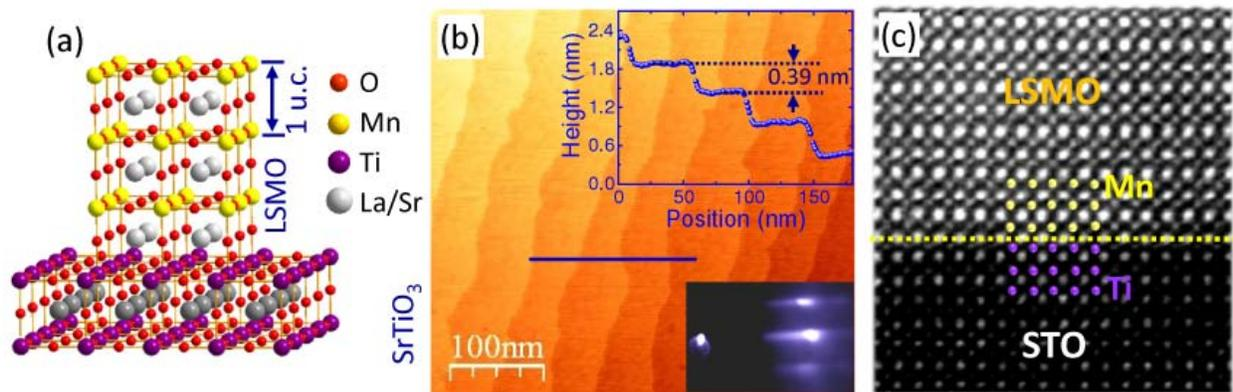
**Figure 1.** Atomically layer-by-layer growth of LSMO on STO (001): (a) Schematic structure model of a 3 unit cell LSMO on perovskite substrate. (b) Surface morphology of a 10 u.c. LSMO thin film on Nb-doped STO imaged by STM ( $V_{\text{tip}} = 2\text{V}$ ,  $I_t = 300\text{ pA}$ ). Inset shows the profile along the blue line. (c) Cross-section STEM image of the LSMO/STO. The film was grown at  $P_{\text{O}} = 80\text{ mTorr}$ .
