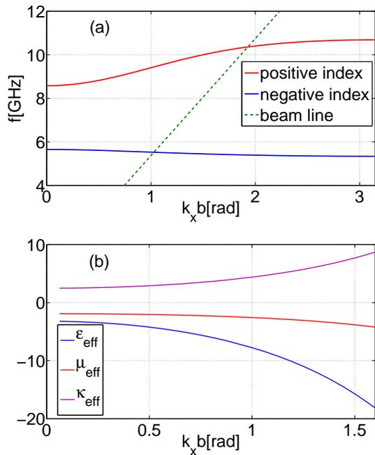
FIG. 3. (Color online) Modes of the NIMW calculated from COMSOL simulations. (a) Dispersion relation for the lowest  $\text{TM}_1$ -like modes (solid lines) and the "beam mode" (dashed line) defined by  $\omega = k_x v_b$ , where  $v_b = 0.9c$ . (b) Extracted effective parameters of the negative index mode.
