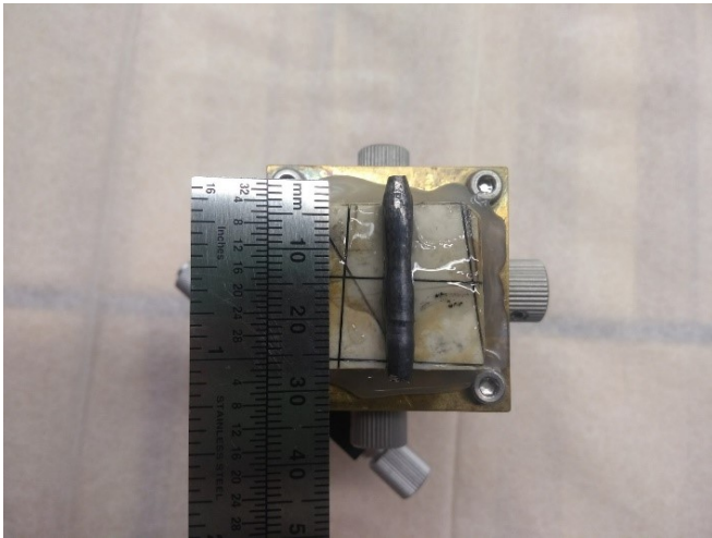
FIG. 5. Single crystal of \text{YbIr}_3\text{Si}_7 grown in a tilting laser diode optical floating zone furnace and mounted onto a three-axis goniometer.
