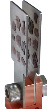
FIG. 8. \text{KYbSe}_2 sample used to measure the field-dependent spin excitations on CNCS. 19 plate-like crystals were coaligned and glued to two aluminum plates with the [1\bar{1}0] direction vertical and the [001] direction orthogonal to the aluminum surface.
