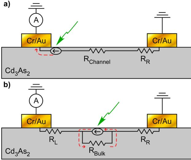
FIG. 5. Circuit model for understanding local CPGE. Equivalent circuit diagrams when circularly polarized photoexcitation is in the vicinity of the contact (a) and away from the contacts (b), respectively. The green arrows indicate the laser position. The red dashed curves indicate the major current flow.
