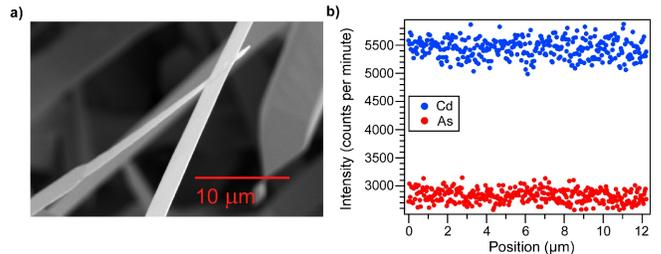
FIG. 6. (a) SEM image of  $\text{Cd}_3\text{As}_2$  nanostructures on an as-grown substrate. (b) Cross section of the EDS spectrum along the nanobelt showing uniform stoichiometry.
