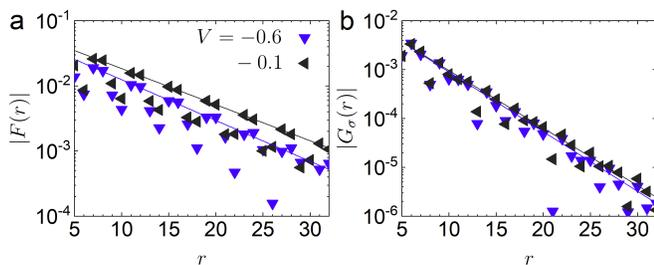
FIG. 5. (Color online) (a) The spin-spin and (b) single-particle correlation functions with electron attraction  $V = -0.6$  and  $V = -0.1$ . The length of cylinder is  $L_x = 64$ . Solid lines denote exponential fit  $F(r) \sim e^{-r/\xi_s}$  and  $G_\sigma(r) \sim e^{-r/\xi_G}$ , where  $\xi_s$  and  $\xi_G$  are corresponding correlation lengths.
