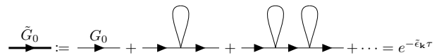
FIG. 2. The geometric series of the 1-loop diagrams defines the “Hartree” renormalized electron propagator.
