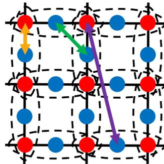
FIG. 1: An illustration of a checkerboard lattice structure representing a metal oxide 2D layer. Red circles represent correlated  $d$  sites (transition metals), and blue circles are non-interacting  $p$  sites (oxygens). The double-arrow lines illustrate examples of bonds used to define the slave-particle operators. The dashed black ellipses indicate the  $d-p-d$  clusters in the layer which overlap with each other on the correlated  $d$ -sites.
