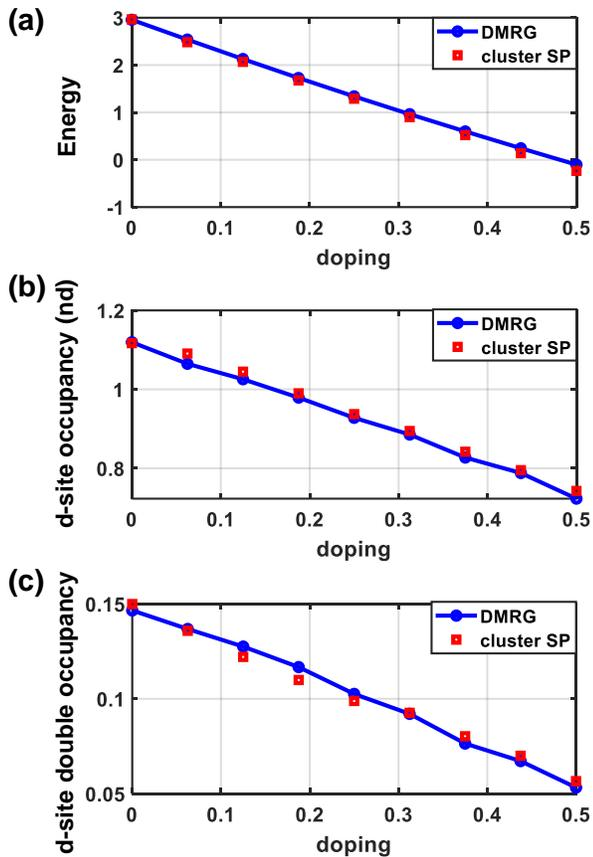
FIG. 7: Panels (a-c) show the total energy of each four-site unit cell (units of  $t$ ),  $d$ -site occupancy, and  $d$ -site double occupancy respectively. They are plotted as functions of the average hole doping level on each  $d$ - $p$  pair. Blue circles represent the DMRG results as benchmarks, while the red squares stand for the cluster SP results assuming a translational period of 4 sites.
