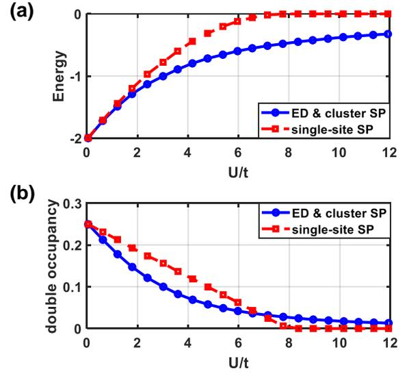
FIG. 3: (a) Total energy and (b) (mean) double occupancy of each site for the half-filled Hubbard dimer as a function of the interaction strength  $U/t$ , where the nearest-neighbor hopping strength  $t$  is the energy unit. Cluster slave-particle (SP) results are identical to the exact diagonalization (ED) results marked by blue circles, while single-site SP results are represented by red squares.
