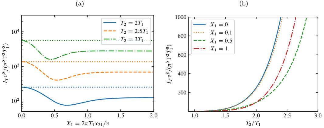
FIG. 11. (Color online) Thermal current between two spin liquids when  $\Gamma_1 = \Gamma_2 = \Gamma$ . (a) Variation with  $X_1$  at a fixed temperature ratio. The broken line shows the value of  $2\langle I_T \rangle_{\Gamma}^{\text{non-int}}$ . (b) Variation with  $n = T_2/T_1$  shows the expected monotonic behavior.
