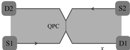
FIG. 2. A single quantum point contact (QPC) is shown, where the two counter-propagating edges of the spin liquid come close and the tunneling between the edge modes takes place as indicated with a dashed line.
