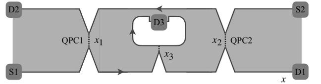
FIG. 7. Fabry-Pérot interferometer with an inner closed edge inside the device. Telegraph noise due to weak tunneling between the bottom edge and the inner edge at  $x_3$  gives an alternative way to probe statistics. As in a Mach-Zehnder device, each tunneling event changes the enclosed topological charge.
