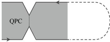
FIG. 5. Geometry, in which the two edges of the spin liquid are treated as spatially separated parts of the same edge. The dashed line shows a long segment, of length  $L$ , connecting the two edges of the interferometer.
