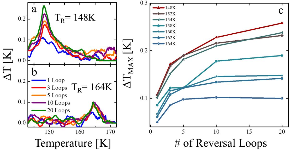
**Figure 3.** Ramp-reversal analysis for different temperatures and number of RLs. a, b)  $\Delta T$  vs.  $T$  at two reversal temperatures (a) 148K and (b) 164K, for different numbers of RLs from one to twenty. Color coding appears in b). c) Maximum value of  $\Delta T$  peak ( $\Delta T_{MAX}$ ) as function of number of RLs for temperatures along the transition. Color coding of temperature appears in figure.
