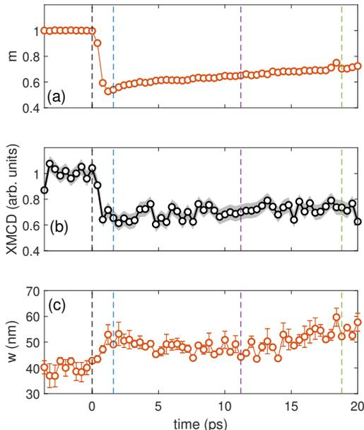
FIG. 7. Evolution of the (a) asymptotic magnetization,  $m(t)$ , and (b) XMCD data obtained when the sample is magnetized with the external field. In panel (b), the error is shown as gray shadow and it is computed from the standard deviation of the pre-pump data. (c) The domain-wall width,  $w(t)$ . The color-coded vertical lines represent the time instances shown in Fig. 6. The domain walls broaden by 31% within the first 2 ps after pumping.
