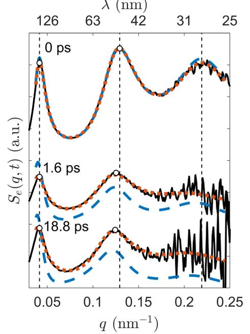
FIG. 11. Data fitting using a fitted Gaussian filter function. The data is presented in the equalized representation of Eq. (2). The experimental data are shown by solid black curves, the empirical fits by dashed red curves, and the fits using a Gaussian filter function, Eq. (C1) by dashed blue curves. Time instances at 0 ps, 1.6 ps, and 18.8 ps are shown and vertically shifted for clarity.
