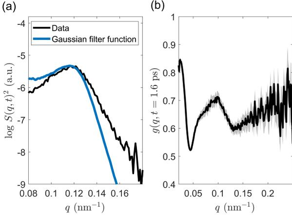
FIG. 14. (a) Comparison of the third-order ring spectrum isolated from experimental data (black curve) and predicted by the use of a suitable Gaussian filter function (blue curve). (b) Time-dependent filter function  $g(q, t)$  computed from experimental data at  $t = 1.6$  ps. The grey shaded area represents the error in determining  $g(q, t)$  from shot noise.
