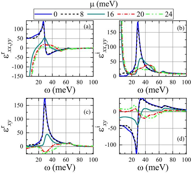
FIG. 4. Permittivity tensor components for the graphene sheet with finite SOC and magnetization. Both the real and imaginary components are shown for several different chemical potentials  $\mu$ . The Zeeman field is set to  $h_z = 20$  meV. From symmetry considerations:  $\epsilon_{xy}(\omega) = -\epsilon_{yx}(\omega)$ , the other off-diagonal permittivity components can be deduced.
