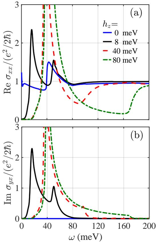
FIG. 2. (Color online). The components of the optical conductivity as a function of frequency. (a) and (b) are the real part of  $\sigma_{xx}(\omega)$  and imaginary part of  $\sigma_{yx}(\omega)$ , respectively. The magnetization is oriented along the  $z$  axis, i.e.,  $\mathbf{h} = (0, 0, h_z)$ . The chemical potential is set to zero,  $\mu = 0$ , and various values of magnetization strength are considered:  $h_z = 0, 8, 40, 80$  meV. The strength of the SOC is set to  $\alpha = 20$  meV.
