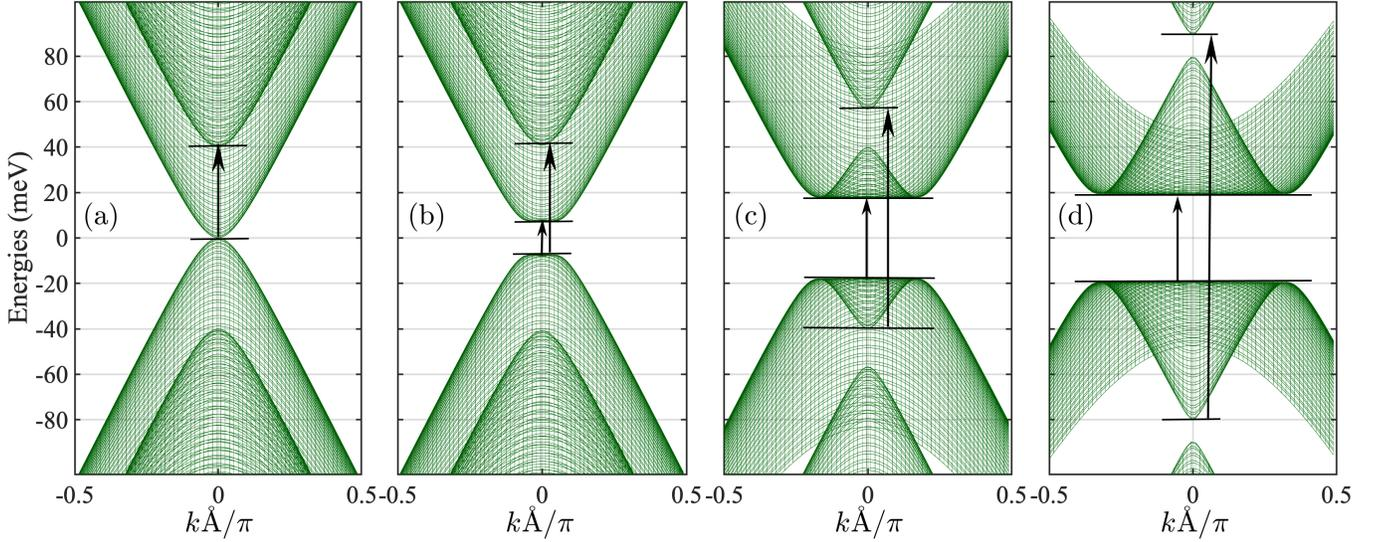
FIG. 3. (Color online). The band structure of graphene in the presence of SOC and magnetization plotted as a function of the normalized momentum  $k\text{\AA}/\pi$ . The chemical potential is set to zero;  $\mu = 0$ , and the strength of the SOC is fixed at  $\alpha = 20$  meV. The magnetization is oriented along the  $z$ -axis and its magnitude increases (from left to right) with the following values (in meV): (a)  $h_z = 0$ , (b)  $h_z = 8$ , (c)  $h_z = 40$ , and (d)  $h_z = 80$ .
