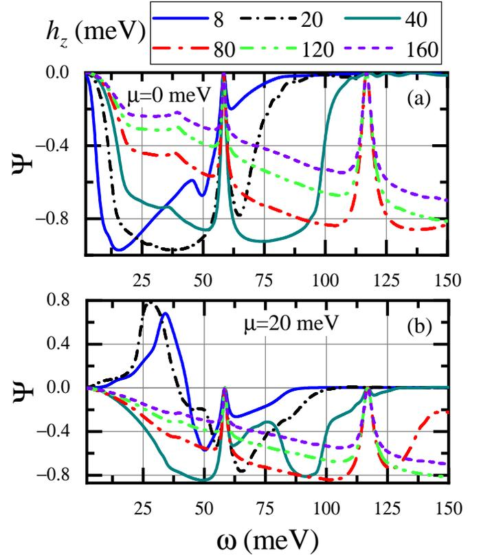
FIG. 6. (Color online). The circular dichroism factor  $\Psi(\omega)$  against the frequency of the incident circularly polarized EM wave. A broad range of magnetizations  $h_z$  at two different values of chemical potential are considered:  $\mu = 0, 20$  meV.
