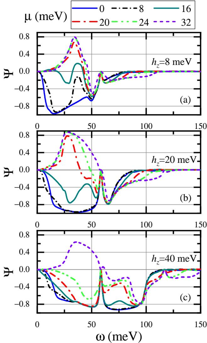
FIG. 5. The circular dichroism  $\Psi(\omega)$  as a function of frequency. Several out-of-plane Zeeman fields  $h_z$  are considered (as shown). Through variations in the gate voltage, the reflected EM energy can exhibit dominant right-handed (positive curves) or left-handed (negative curves) behavior.
