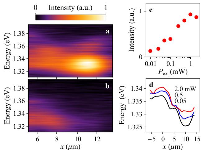
FIG. 3: **Excitation power dependence of IX propagation.** (a,b)  $x$ -energy images of IX luminescence in the drain region for  $P_{\text{ex}} = 2$  mW (a) and  $0.05$  mW (b). (c) Total IX luminescence intensity in the drain (integrated over  $x = 6 - 13 \mu\text{m}$ ) vs  $P_{\text{ex}}$ . (d) IX energy vs position for  $P_{\text{ex}} = 0.05$  (black),  $0.5$  (blue), and  $2$  (red) mW. For all data,  $V_g = 10$  V,  $T = 1.7$  K.
