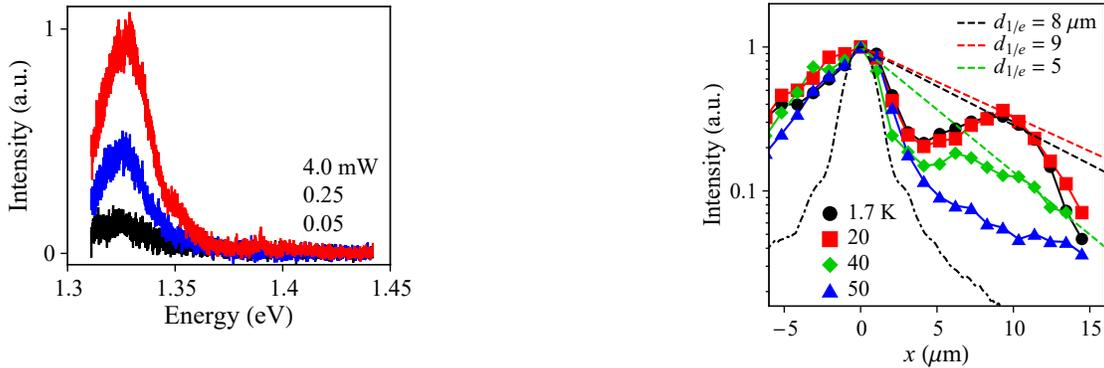
FIG. 9: **Excitation power dependence.** Luminescence spectra of propagating IXs at  $x = 10 \mu\text{m}$  for  $P_{\text{ex}} = 0.05, 0.25,$  and  $4 \text{ mW}$ . Excitation spot is at  $x = 0$ ,  $V_g = 10 \text{ V}$ ,  $T = 1.7 \text{ K}$ .
