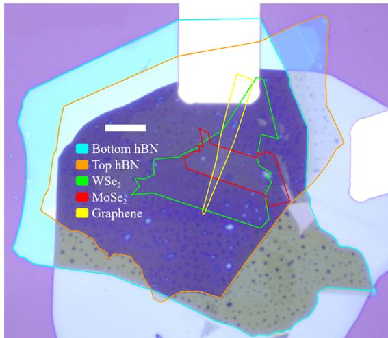
FIG. 7: **The layer pattern.** Microscope image showing the layer pattern of the device on an area larger than in Fig. 1b. Scale bar is  $10 \mu\text{m}$ . The green, red, yellow, cyan, and orange lines indicate the boundaries of  $\text{WSe}_2$  and  $\text{MoSe}_2$  monolayers, graphene gate, and bottom and top hBN layers, respectively.
