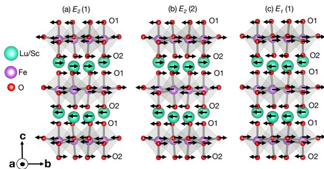
FIG. 5. Atomic displacements that contribute to the Raman active  $E_2(1)$ ,  $E_2(2)$ , and  $E_1(1)$  modes computed at zero pressure for the ground state  $P6_3cm$  structure of  $\text{LuFeO}_3$  and  $\text{ScFeO}_3$ . The atomic displacement patterns of  $\text{Lu}_{0.6}\text{Sc}_{0.4}\text{FeO}_3$  are qualitatively similar, as the primary effect of the mixed Lu/Sc composition is a change in mass.
