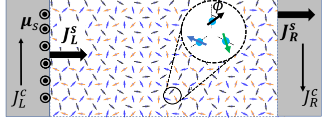
FIG. 2. A nonlocal measurement setup containing normal metal/nAFM/normal heterostructure. A charge current in the left layer generates a spin accumulation \mu_s via spin Hall effect, which injects a spin current into nAFM layer. The spin current mediated by the collective modes in the middle layer passes the second interface by virtue of spin pumping effect. The pumped spin current is measured in the right layer via the inverse spin Hall effect.
