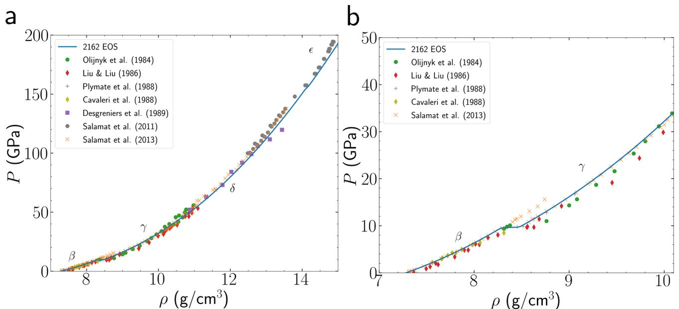
FIG. 7. Room temperature isotherm for the 2162 EOS with a comparison to experimental data over (a) the full range of experimental data and (b) near the  $\beta$ - $\gamma$  phase transition. Experimental data are from Refs. 23–29.
