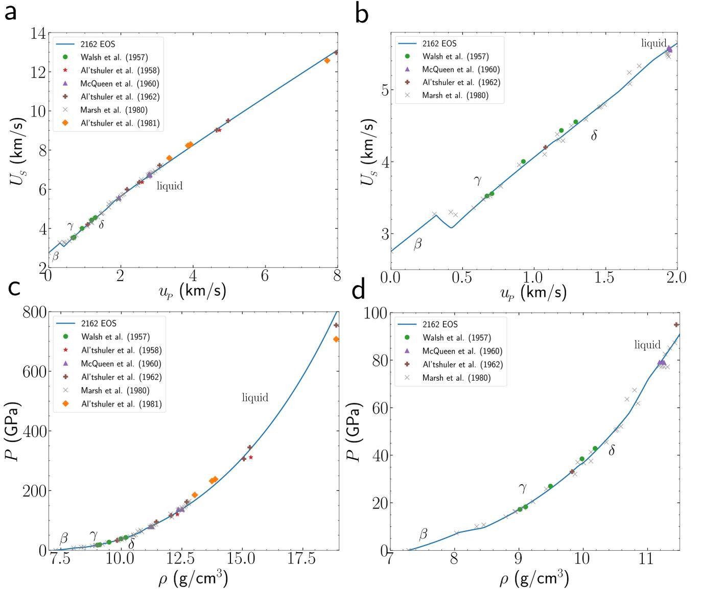
FIG. 8. Comparison of the 2162 EOS to shock experiments along the principal Hugoniot. The  $U_s$ - $u_p$  relations are shown over (a) a wide range of shock speeds including the liquid phase and (b) over a narrow range of shock speeds focusing on the solid phases. The pressure  $P(\rho)$  along the Hugoniot is shown over (c) a wide range of pressure and (d) a narrow range of pressure focusing on the solid phases. Experimental data are from Refs. 33–38.
