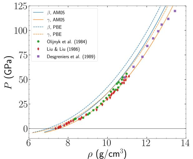
FIG. 1. Cold curves for the  $\beta$  (blue) and  $\gamma$  (orange) phases of tin using the AM05 (solid lines) and PBE (dashed lines) exchange-correlation functionals. Experimental DAC data are from Refs. 23–25.
