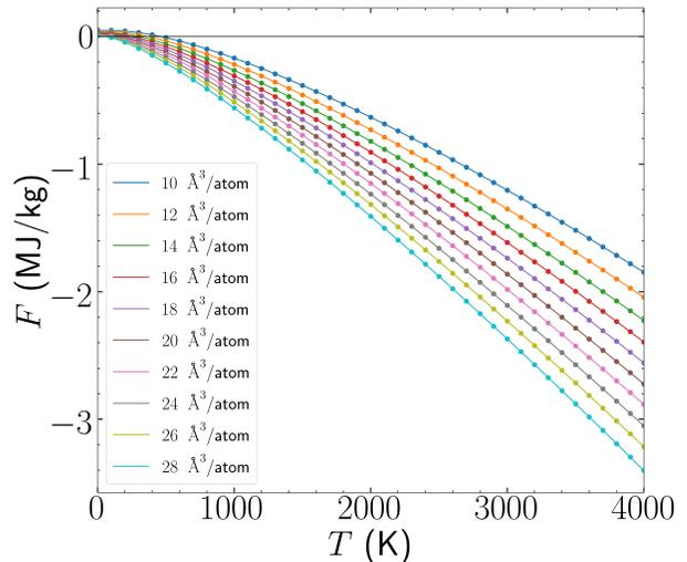
FIG. 3. Free energy as a function of temperature for the  $\gamma$  phase computed from phonon calculations (dots) and the corresponding Debye model fit (lines) using Eq. 9 over a range of different volumes.
