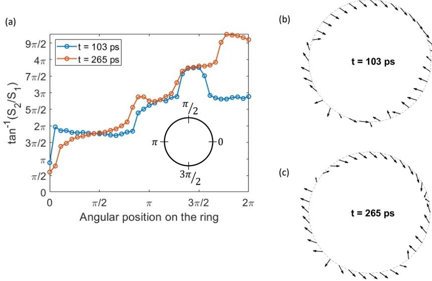
FIG. 5. (a) The direction pointed by the linearly polarized Stokes vector  $S_1\hat{x} + S_2\hat{y}$  around the ring at two time instances. The angle  $\tan^{-1}(S_2/S_1)$  has been unwrapped in the range  $[0, 6\pi]$ . (b) and (c) show the linearly polarized Stokes vector in the ring at  $t = 103$  ps and  $t = 265$  ps respectively.
