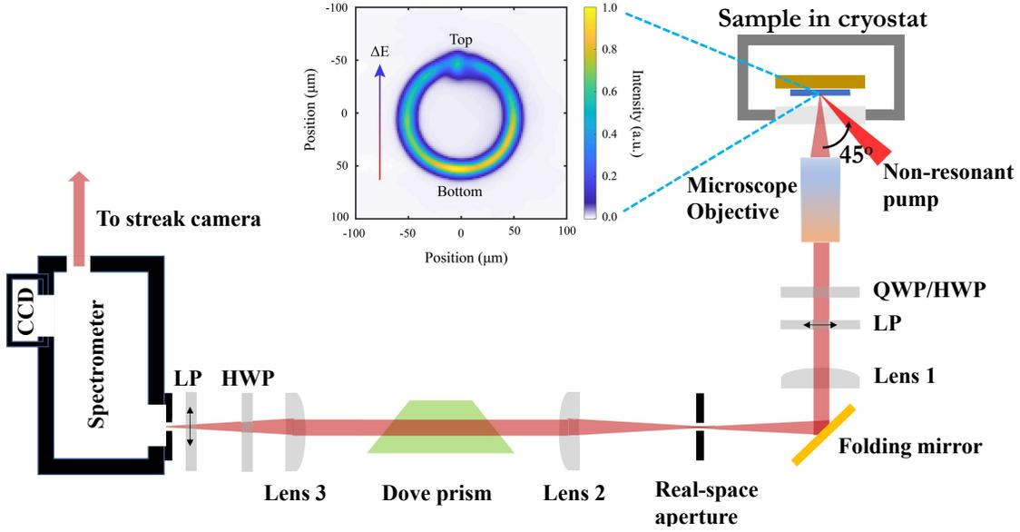
FIG. 1. Schematic of the experimental setup. Inset shows a time integrated image of the photoluminescence from the ring microcavity also showing the direction of the cavity gradient  $\Delta E$ . QWP: quarter waveplate, HWP: half waveplate, LP: linear polarizer.
