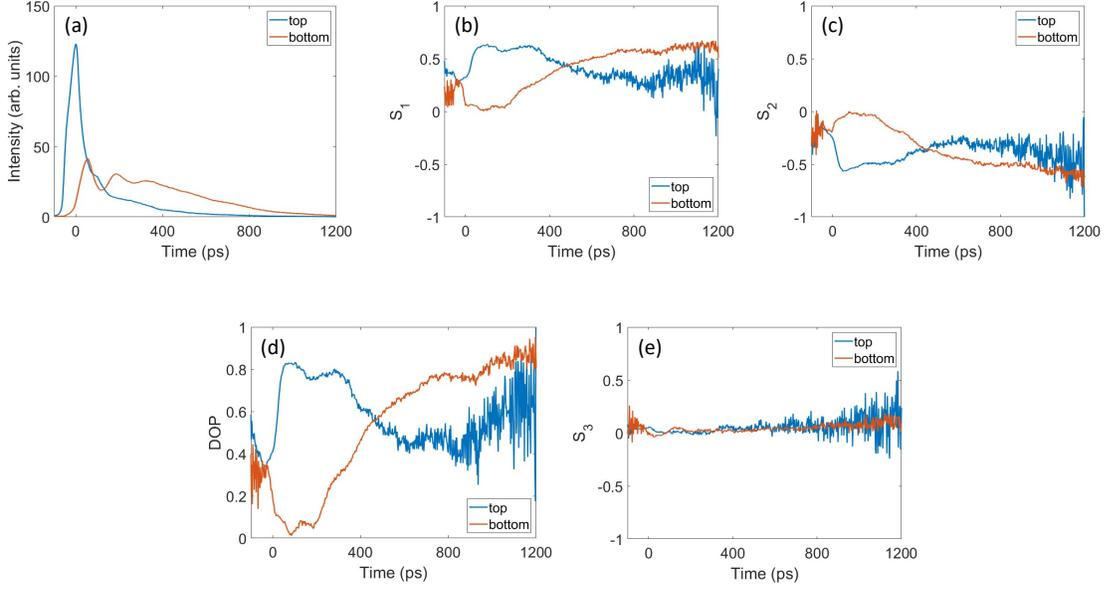
FIG. 3. Comparison of the polarization between the top and bottom of the ring as a function of time. Degree of polarization (DOP) is given by  $\sqrt{S_1^2 + S_2^2 + S_3^2}$ .
