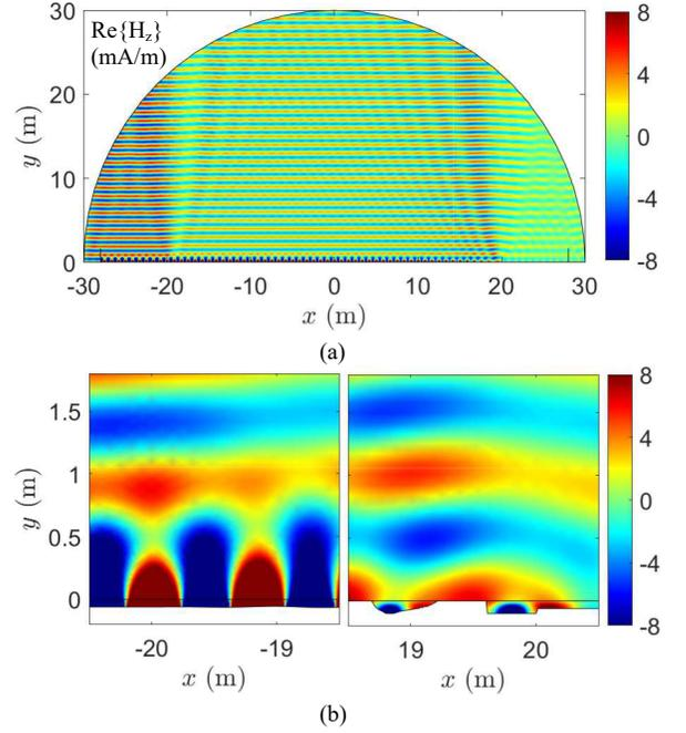
FIG. 8. PW-to-SW conversion characteristics of the  $40\lambda$ -long thickness-modulated grounded substrate metasurface at  $f = 300$  MHz. A unit-amplitude TM-mode plane illuminates the surface from the direction  $\phi^i = 90.2^\circ$ . (a) Snapshot of the total magnetic field  $H_z(x, y)$ . (b) Magnified views of  $H_z(x, y)$  over the transition regions of the metasurface coupler near  $x = -20$  m (left) and  $x = 20$  m (right).
