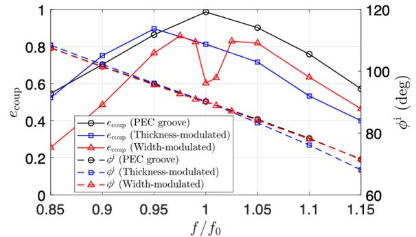
FIG. 11. The coupling efficiency and the associated direction of incidence with respect to the normalized frequency for the three  $40\lambda$  physical coupler designs.
