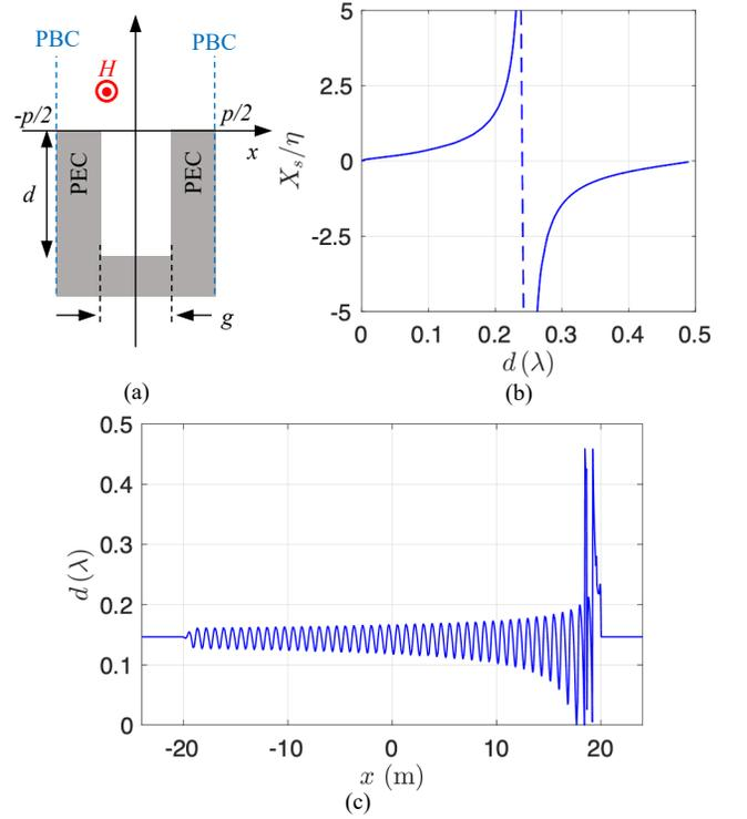
FIG. 5. PEC groove array metasurface design. (a) A unit cell having a rectangular groove of dimensions  $g \times d$  in a PEC ground in the  $xz$ -plane. (b) Design curve for the surface reactance at  $y = 0$  with respect to  $d$  using  $p = \lambda/20$  and  $g = p/2$ . (c) The depth distribution for the PEC groove array metasurface along the  $x$ -axis.
