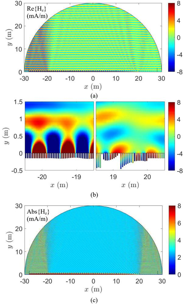
FIG. 6. PW-to-SW conversion characteristics of the  $40\lambda$ -long PEC groove array metasurface. The design frequency is  $f = 300$  MHz. A unit-amplitude TM-mode plane illuminates the surface from  $\phi^i = 90.19^\circ$ . (a) Snapshot of the total magnetic field  $H_z(x, y)$ . (b) Magnified views of  $H_z(x, y)$  near the edges of the metasurface coupler, i.e.,  $x = -20$  m (left) and  $x = 20$  m (right). (c) The magnitude distribution of the  $H_z(x, y)$ .
