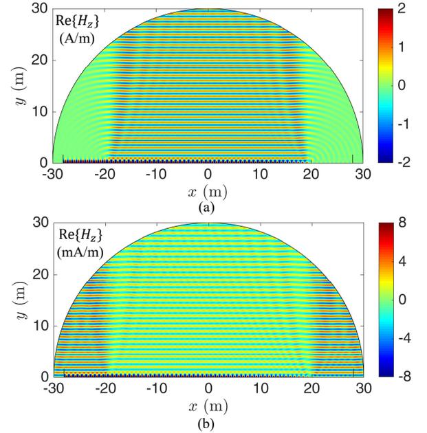
FIG. 4. Spatial field distributions of the  $40\lambda$ -long coupler design. (a) Snapshot of  $H_z(x, y)$  when the surface is operated as a transmitting LWA. The surface is excited by a TM SW with an incident power of 7.298 kW/m. (b) Snapshot of  $H_z(x, y)$  when the surface is operated as a PW-to-SW coupler. An  $x$ -polarized unit-amplitude plane wave illuminates the surface at normal incidence.
