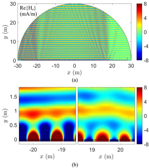
FIG. 10. PW-to-SW conversion characteristics of the  $40\lambda$ -long width-modulated dielectric ridge metasurface at  $f = 300$  MHz. A unit-amplitude TM-mode plane wave illuminates the surface from the  $\phi^i = 90.21^\circ$ . (a) Snapshot of the total magnetic field  $H_z(x, y)$ . (b) Magnified views of  $H_z(x, y)$  near the metasurface coupler edges at  $x = -20$  m (left) and  $x = 20$  m (right).
