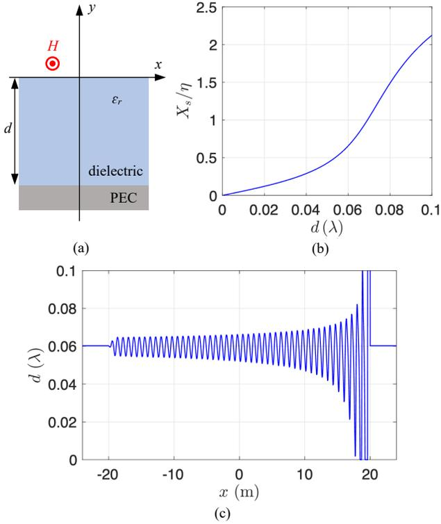
FIG. 7. Thickness-modulated grounded dielectric substrate metasurface design. (a) A dielectric substrate of thickness  $d$  and a relative permittivity  $\epsilon_r$  on a PEC ground. (b) Design curve for the surface reactance at  $y = 0$  with respect to  $d$  when  $\epsilon_r = 11$ . (c) The thickness distribution of the  $40\lambda$ -long thickness-modulated dielectric substrate metasurface.
