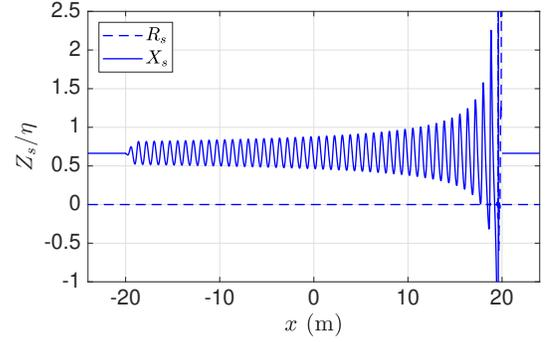
FIG. 3. The surface impedance  $Z_s$  for the  $40\lambda$ -long uniform-aperture LWA normalized by  $\eta$ .
