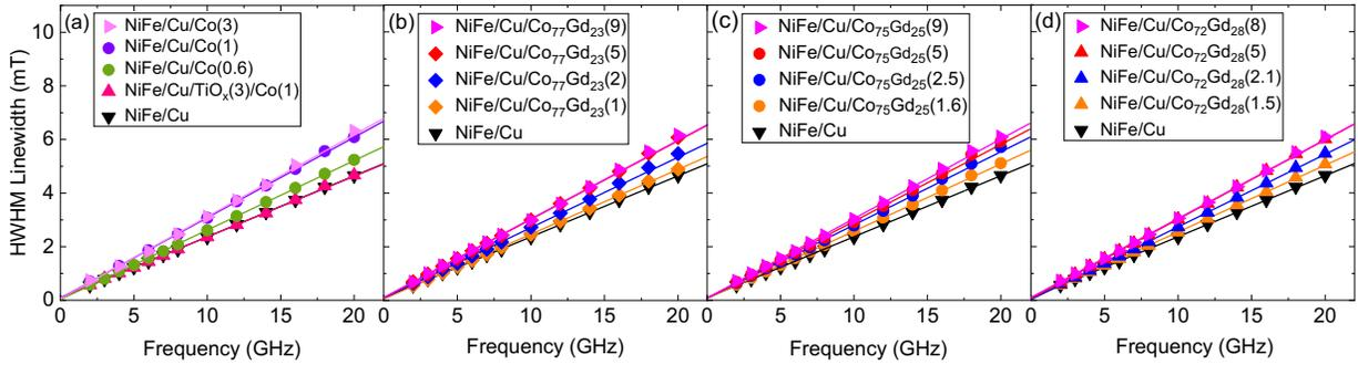
187 **FIG. 3.** (a) Half-width-at-half-maximum (HWHM) FMR linewidth versus frequency for stacks with a spin
