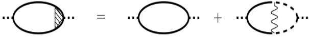
FIG. 2. Feynman diagrams defining the vertex corrections through the Ward identity. The thick solid (dashed) lines are the interacting (non-interacting) Green functions. The shaded triangle denotes vertex corrections arising from electron correlations. The dotted lines denote a generic external momentum transfer into and away from the pair bubble.
