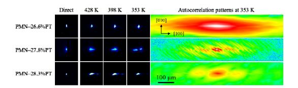
FIG. 3. Speckle patterns for PMN–26.6%PT, PMN–27.8%PT, and PMN–28.3%PT samples. Direct beam patterns are also shown for reference. Autocorrelation patterns at 353K are shown to the right side of speckle patterns.
