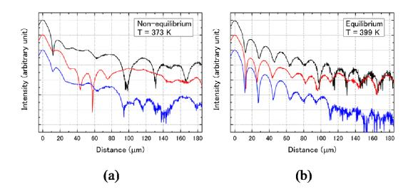
FIG. 6. Shot by shot cross-section profiles. Shot by shot fluctuation of the domain boundaries are shown. (a) Fluctuation of domain boundaries are clearly shown at non-equilibrium condition. (b) No obvious fluctuation could be recognized at equilibrium condition.
