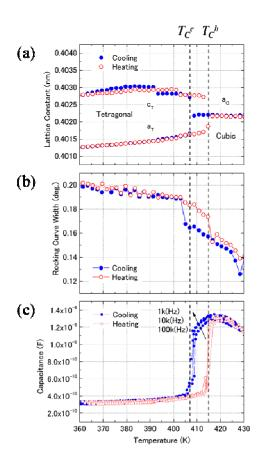
FIG. 4. Temperature dependences of (a) the lattice constant, (b) the rocking curve width (FWHM) at the 200 Bragg peak position, and (c) the capacitances for each frequency for the PMN–27.8%PT sample.
