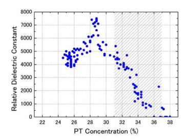
FIG. 1. PMN–x%PT dielectric constants depend on the Ti concentration. This graph was reconstructed from Fig. 7 in Ref. 19. The MPB region is indicated by the hatched area
