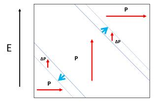
Fig. 7. Schematic model of antiphase shift of domain walls under application of electric field. Elastic strain is almost preserved at the antiphase shift of domain walls
