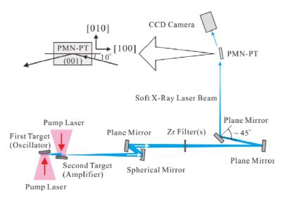
FIG. 2. Schematic of the experimental setup and temperature dependences of the coherent SXR speckle patterns. The polarized coherent SXR laser beam is focused on the sample surface, and the reflected beam from the sample is acquired by an SXR CCD camera.
