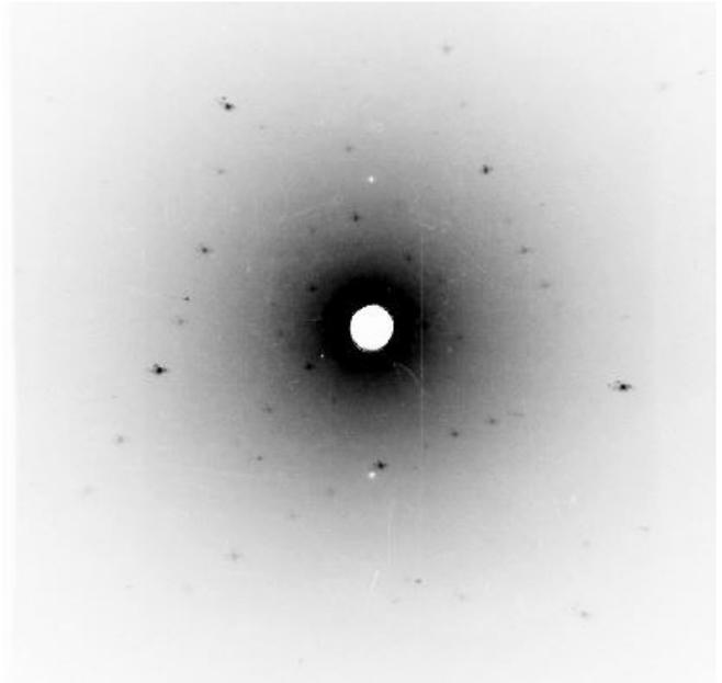
FIG. 6. Laue x-ray diffraction pattern of the sample confirms it is a single crystal, the  $\text{Cu}_{94}\text{Mn}_6$  cube sample was etched in 15% nitric acid. The 6 at.% Mn concentration was estimated from scaling using the observed temperature ( $T_g = 31.5$  K) at which the remanence disappeared.
