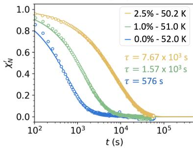
FIG. 7. The value of  $\chi'(t)$  measured in the 2.5%, 1.0% and 0.0% samples is plotted over an extended measurement time of 20 hours. The data was fitted using the stretched exponential function, with fitted lifetime shown.
