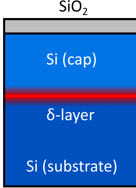
FIG. 2. The composition of samples under investigation. The \delta -layers (red) are deposited on a silicon substrate (dark blue), upon which an additional layer of silicon (light blue) is deposited. This “cap” frequently contains significant impurity/defect density and will be modeled as such. On top of the stack a thin layer ( \sim 2\text{nm} ) of \text{SiO}_2 (grey) forms, the thickness of which varies slightly from sample to sample.
