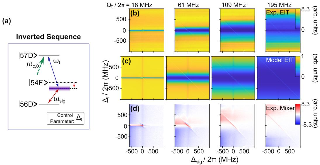
Stark effects from nearby transitions can interfere with signal detection. The mixer data at  $\Omega_t/2\pi = 195$  MHz also cautions that the Raman peak-based tuning scheme shown here is approximately of comparable magnitude as the nonresonant background arising from the AC Stark effect.
