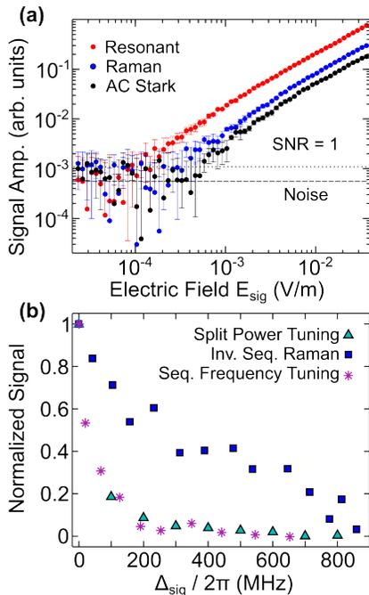
FIG. 7. (a) Comparison of the baseline sensitivity of on-resonance detection on the 56D-54F transition, the Raman EIT peak, and the AC stark shift at 21.5 GHz. (b) Roll-off of the mixer signal for the different tuning mechanisms: Split scheme power tuning (cyan triangles), sequential scheme frequency tuning (magenta stars), and inverted sequence Raman peak-based frequency tuning (blue squares).
