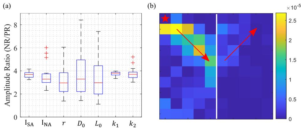
FIG. 6. (a) The sensitivity test for system parameters, shown as a boxplot. 20 numerical simulations at small signal frequency  $f = 18.5$  Hz are used for each parameter study. (b) The experimental results of the system excited from the top-left corner instead of the bottom left. The average kinematic energy is plotted.
