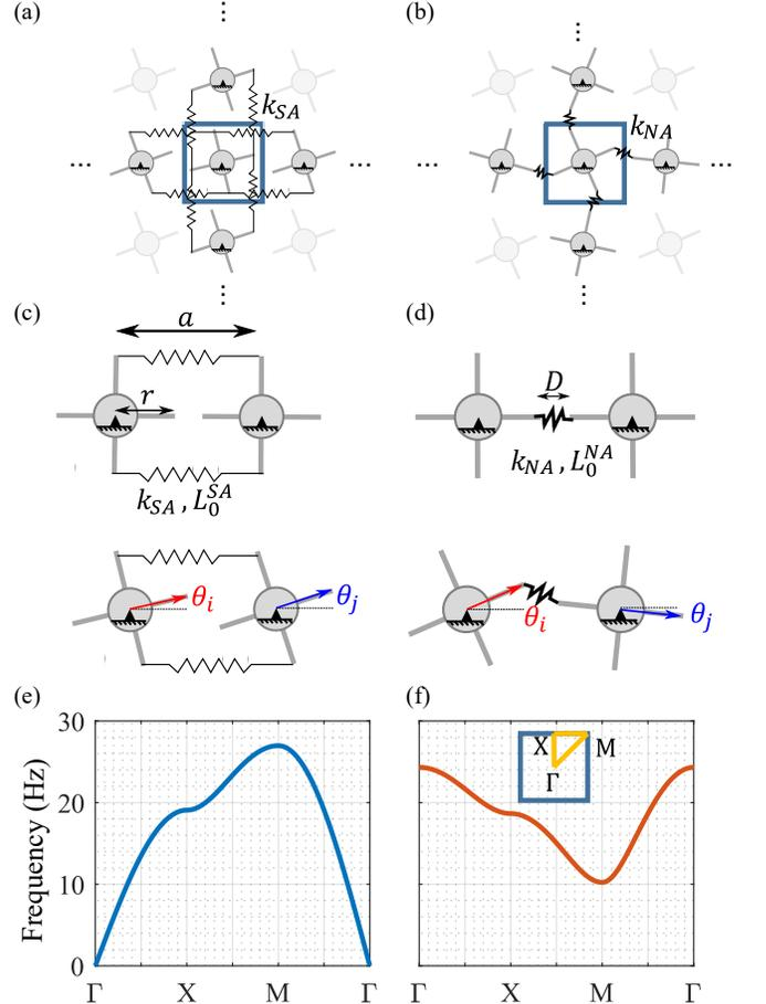
FIG. 1. Schematics of SA type (a) and NA type (b) rotator lattice structures. The blue square identifies the unit cell. (c) The detailed view of the SA inter-rotator connection. (d) The detailed view of the NA inter-rotator connection. (e) SA lattice linear dispersion relation. (f) NA lattice linear dispersion relation.
