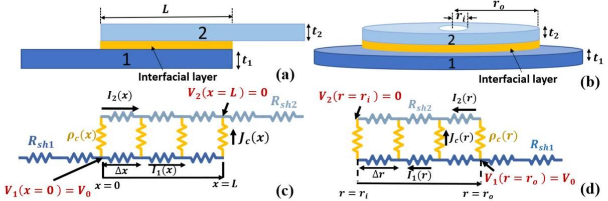
**Figure 2.** Electrical contact between two contacting members in (a) Cartesian, (b) circular geometry. (c), (d) its corresponding transmission line model. In (a) and (b), a thin interface layer (ohmic, Schottky, or tunneling type) is sandwiched between the two contacting members. The thicknesses of thin film 1 and 2 are  $t_1$  and  $t_2$ , respectively.
