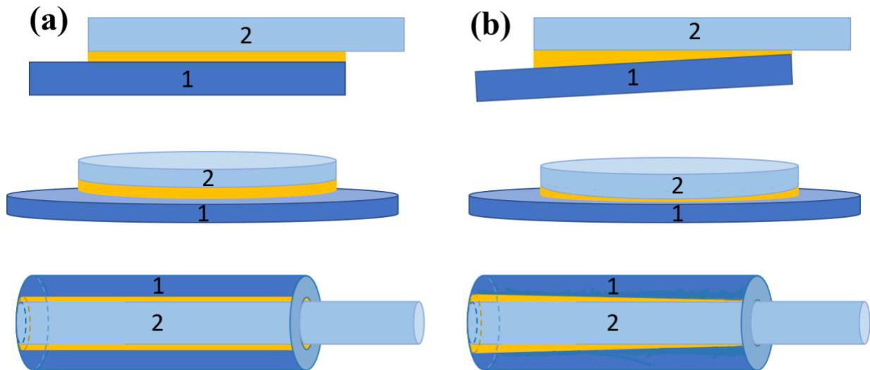
**Figure 1.** Electrical contact between contact member 1 and 2 for different electrode geometry.
